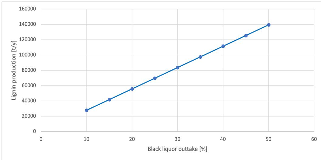
**Figure 4.3:** Produced lignin from the model with supply of 320 kg CO<sub>2</sub>/ton lignin and 255 kg H<sub>2</sub>SO<sub>4</sub>/ton lignin.
