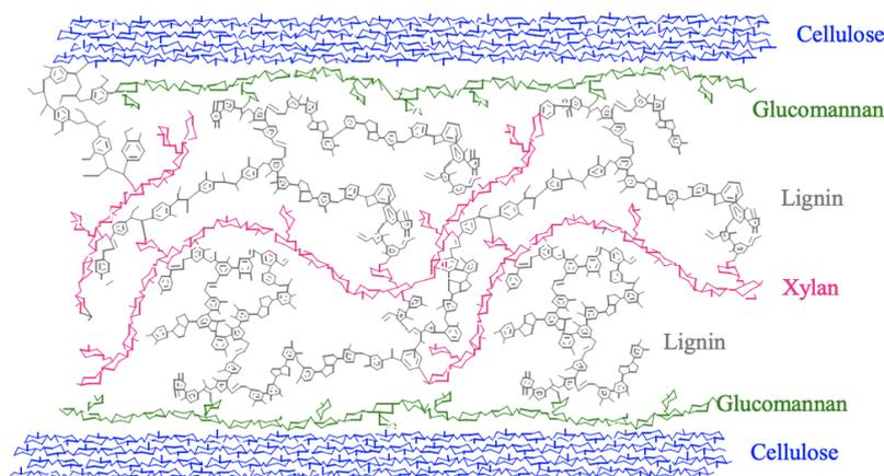
**Figure 2.1:** Distribution of cellulose, hemicellulose, and lignin on a molecular level [1].
