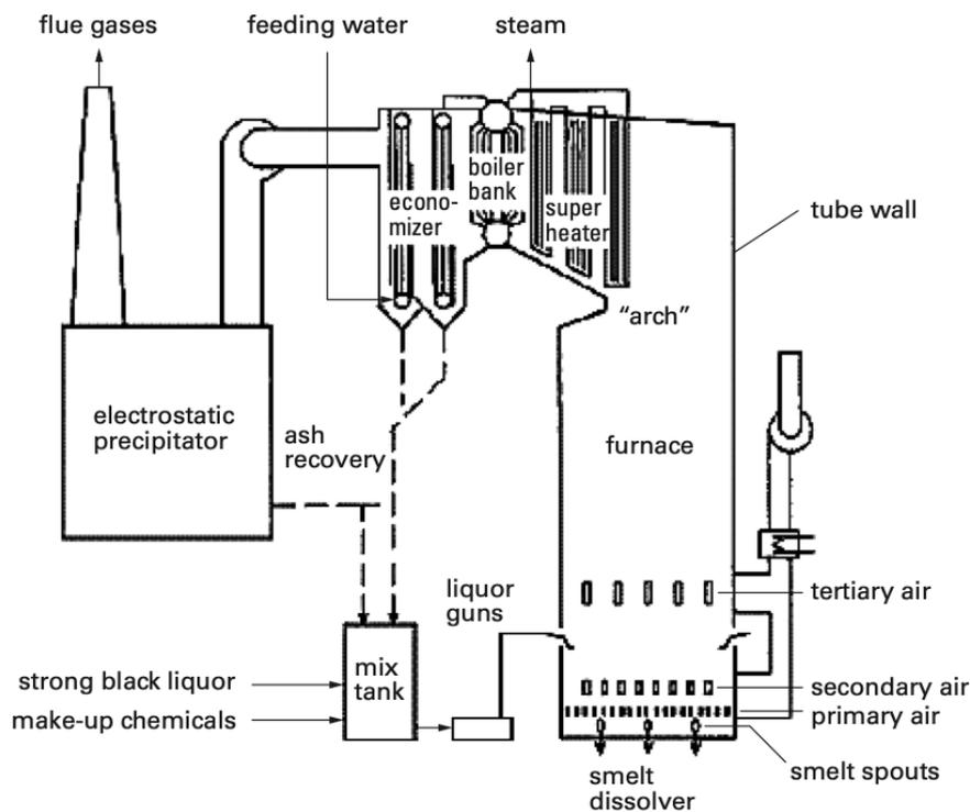
**Figure 2.6:** A visual description of the recovery boiler [6].
