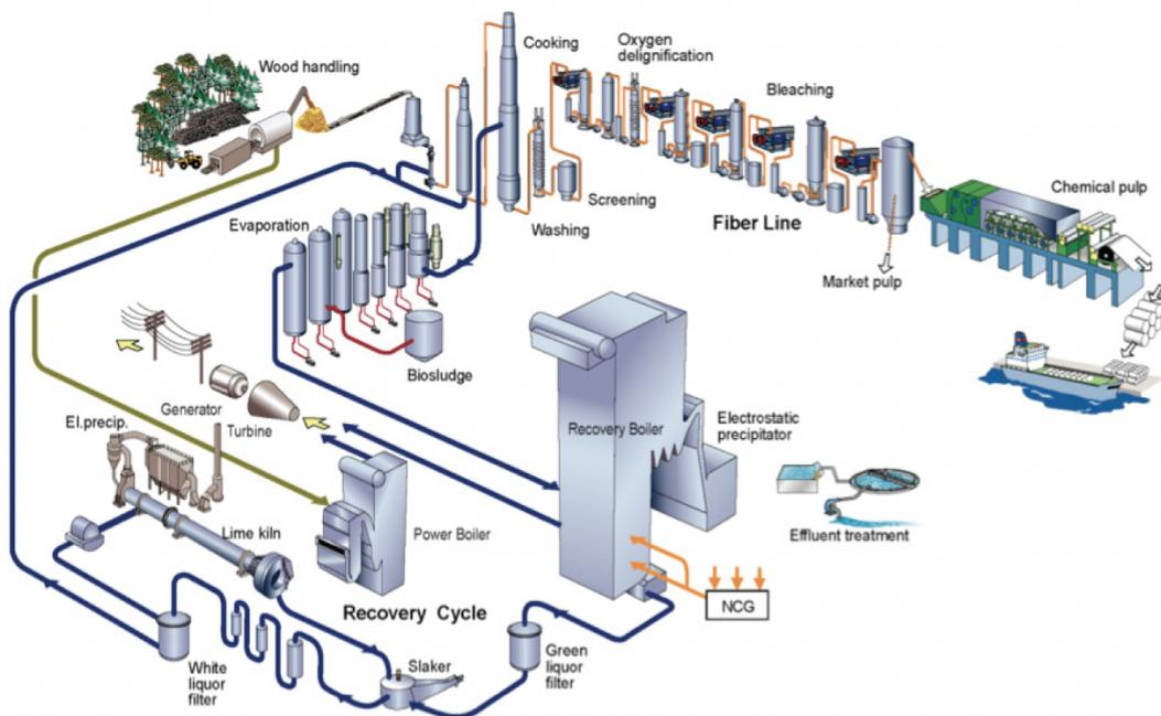
Figure 2.4: Overview of each step of a conventional pulp mill [4].
