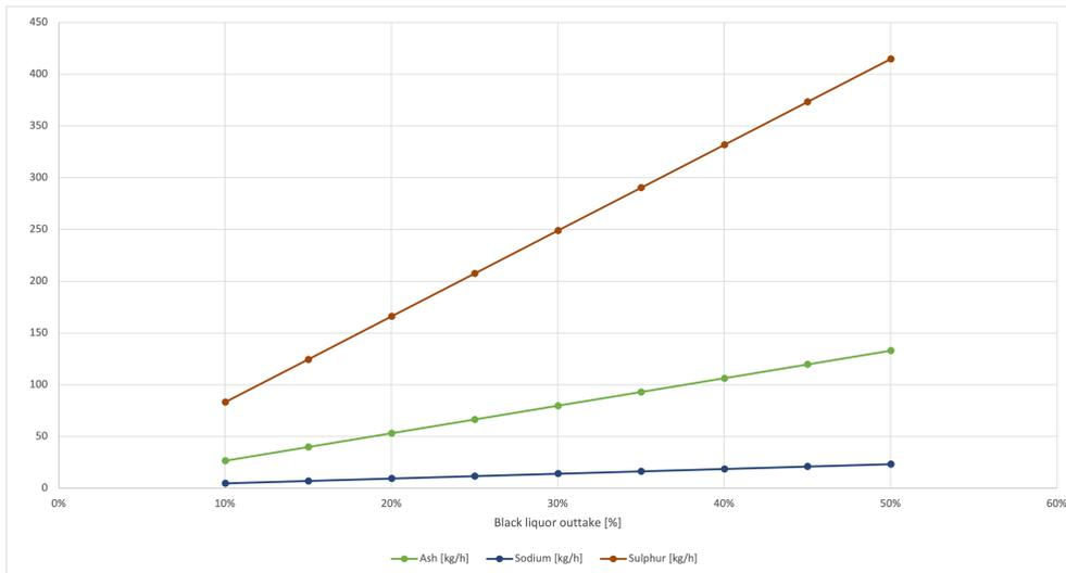
**Figure 4.5:** Ash, sodium, and sulphur content in the final lignin with 320 kg CO<sub>2</sub>/ton lignin and 255 kg H<sub>2</sub>SO<sub>4</sub>/ton lignin.
