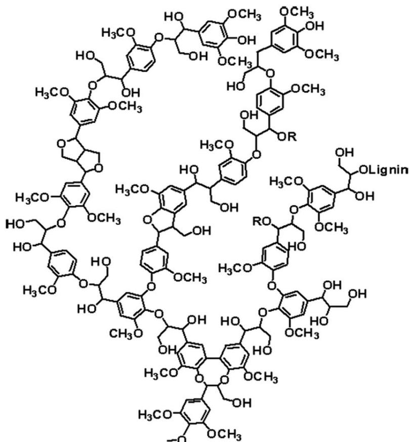
**Figure 2.3:** Chemical structure of an example of how the macromolecule lignin can look like [3].
