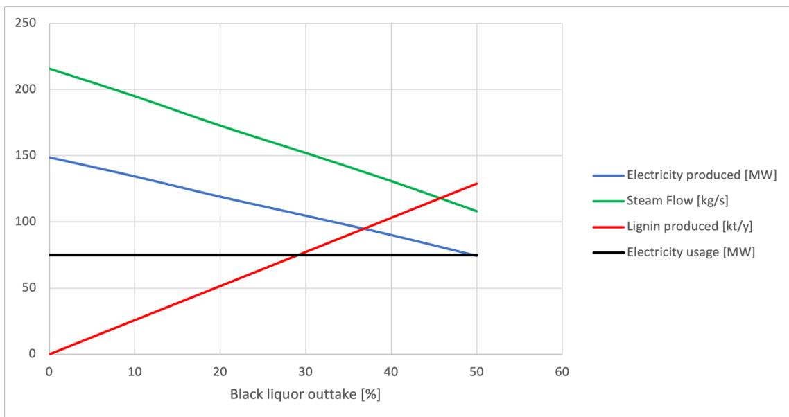
**Figure 4.7:** Steam, electricity and lignin produced in relation to black liquor outtake. The black line indicates the electricity usage of the mill.
