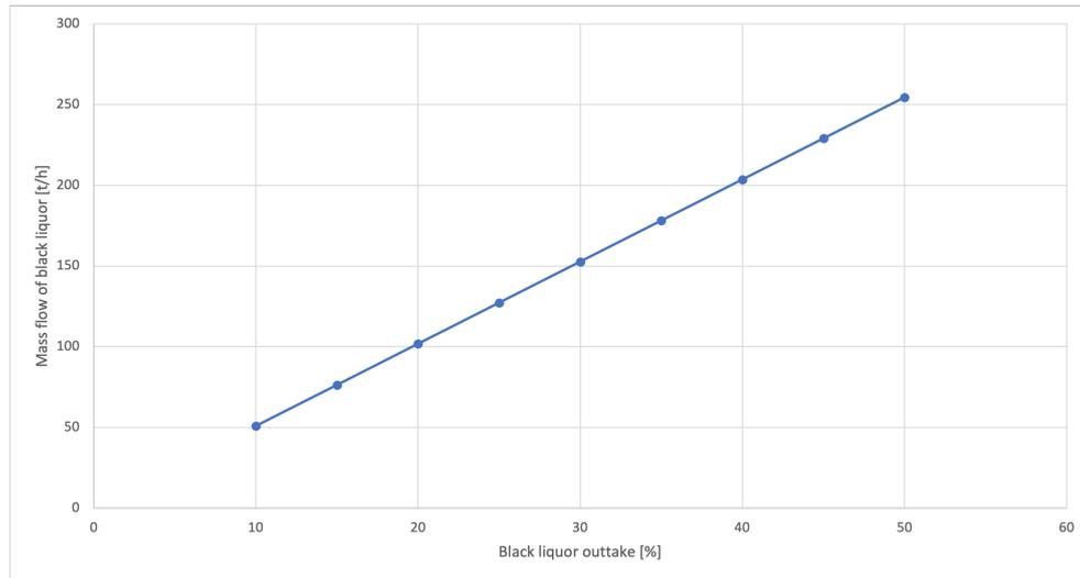
**Figure 4.2:** Amount of black liquor going into the lignin recovery boiler with different percentages of black liquor extraction.
