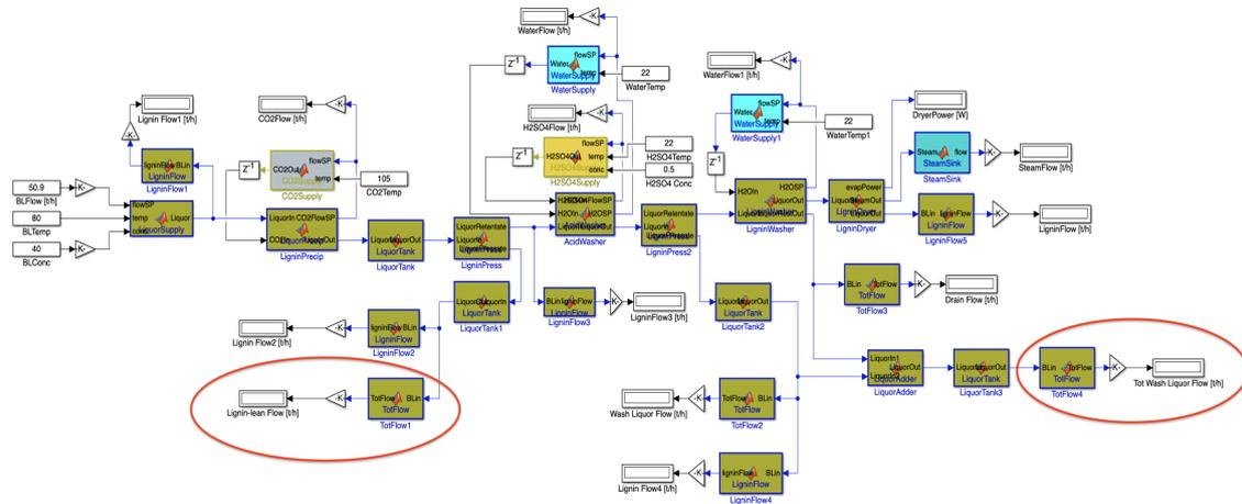
**Figure 4.1:** The Simulink model showing with red circles where the filter presses and water flows are changed.
