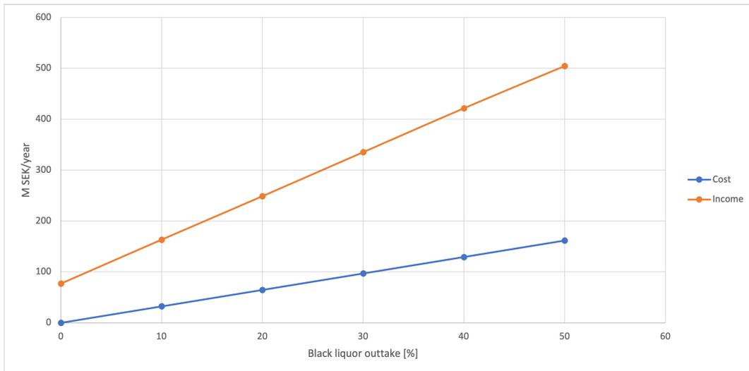
**Figure 4.8:** Incomes and costs of the lignin recovery plant.
