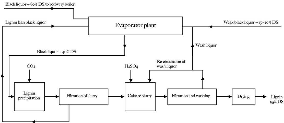
**Figure 2.7:** A schematic view of the lignin removal process.
