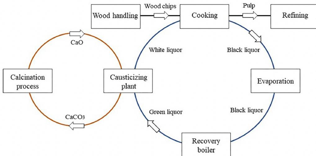
**Figure 2.5:** The chemical recovery cycle in a kraft process [5].
