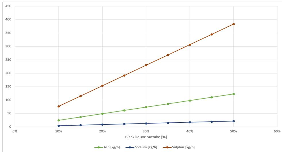
**Figure 4.6:** Ash, sodium, and sulphur content in the final lignin with 220 kg CO<sub>2</sub>/ton lignin and 175 kg H<sub>2</sub>SO<sub>4</sub>/ton lignin.
