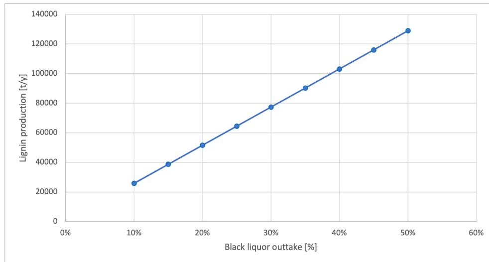
**Figure 4.4:** Produced lignin from the model with supply of 220 kg CO<sub>2</sub>/ton lignin and 175 kg H<sub>2</sub>SO<sub>4</sub>/ton lignin.
