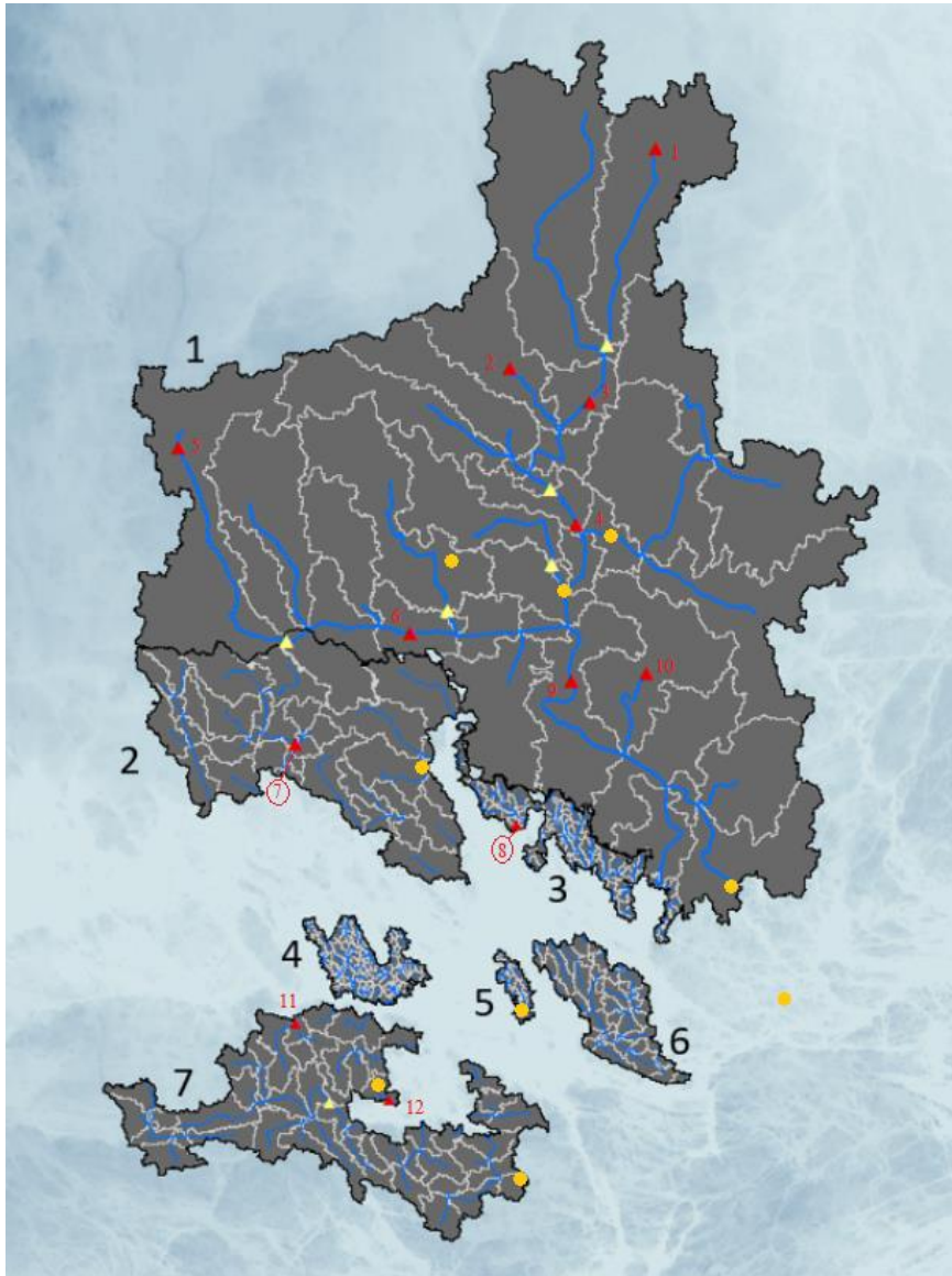
Figure 5. SWAT models in a collected representation. Red triangles represent WWTPs, yellow triangles represent flow gauges, and orange circles represent meteorological stations. WWTPs also have numbers colored with red, connected to the WWTPs listed in Table 10. Numbers colored with black show the different models. In this report model 1 is named Stäket, model 2 Enköping, model 3 Stäket Under, model 4 Strängnäs Island, model 5 and 6 Ekerö, and model 7 Strängnäs.
