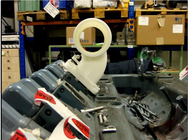
Figure 10-13 - The rapid prototype model of the Budget Viper intake manifold
