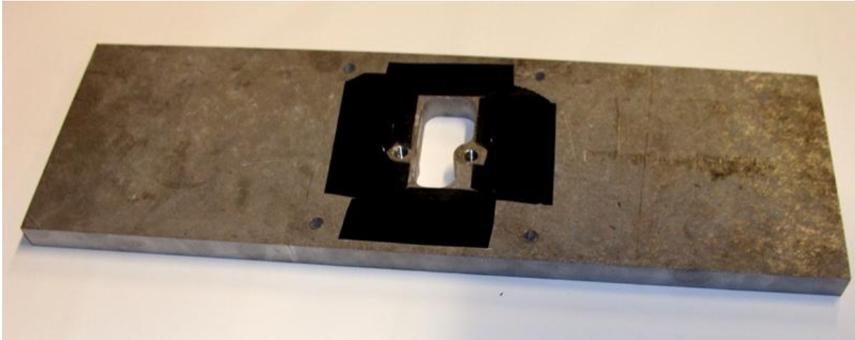
Figure 4-4 – Fixture plate between intake manifold and flow bench. The black tape on around the port hole is used as a seal to prevent leakage.
