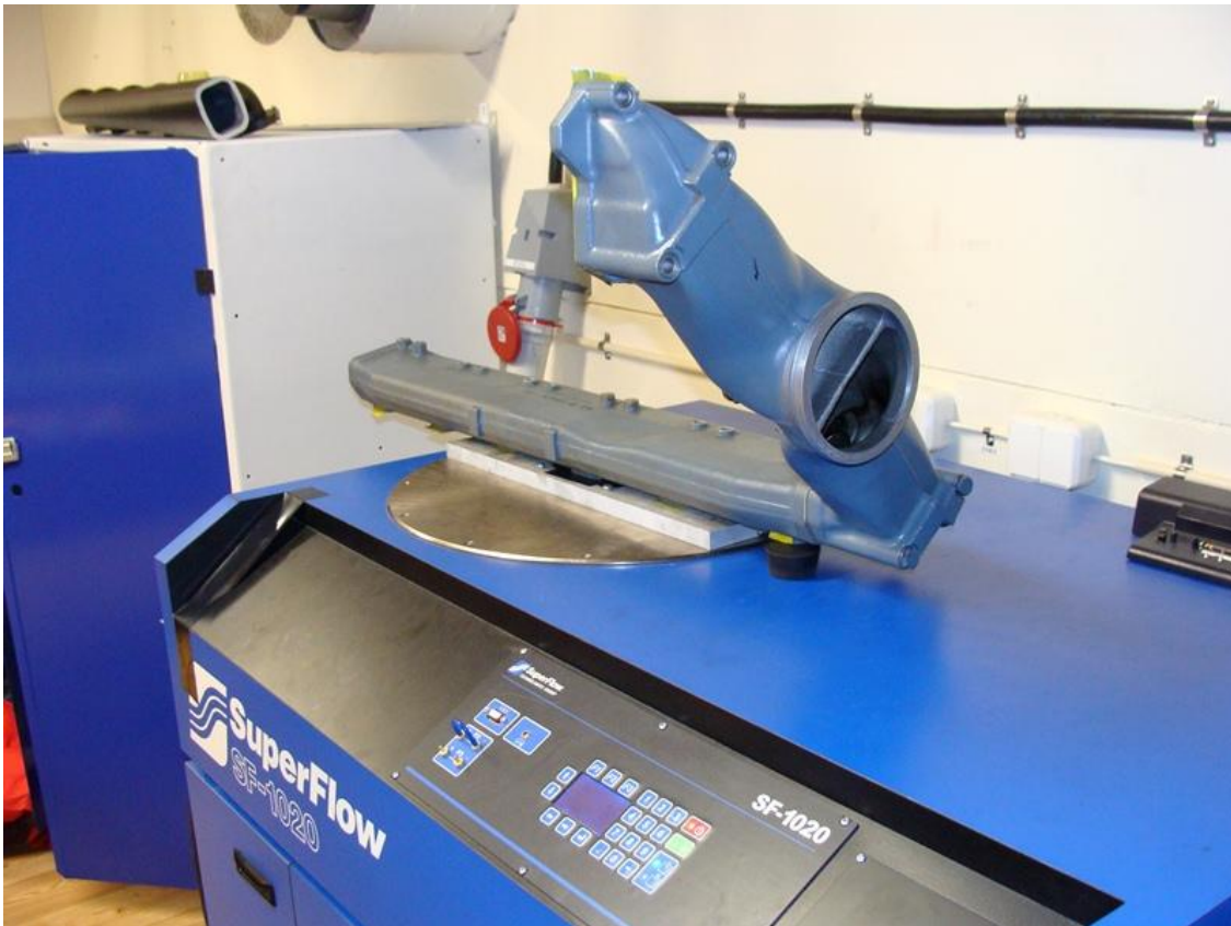
Figure 4-5 – Flow test of cylinder port number 9 in the flow bench. The bench is set to have 25 inch water below ambient pressure and is hence sucking in air through the big inlet hole.
