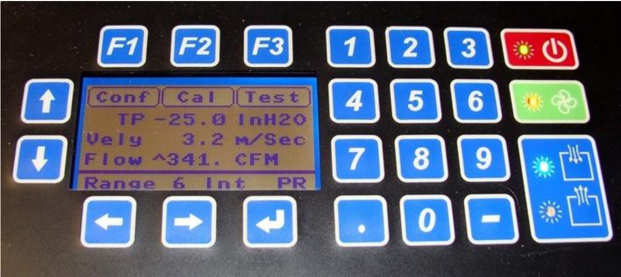
Figure 4-3 – The flow bench display
