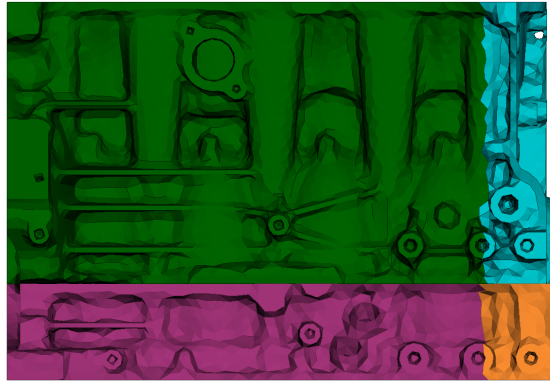
Figure 3.1: The top right hand, in blue colour, and the bottom right hand, in orange colour, illustrate the block side and the bed plate side, respectively.
