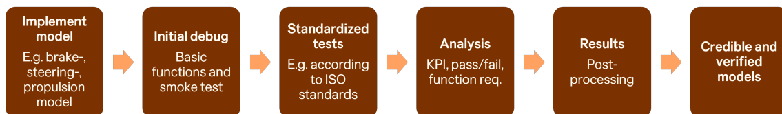
Figure 4.1: The resulting flowchart of the Virtual Verification Framework for Motion Systems.
