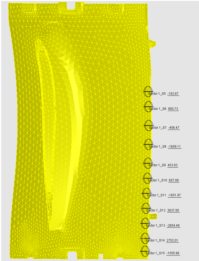
Figure 11 Resulting forces in the support points
