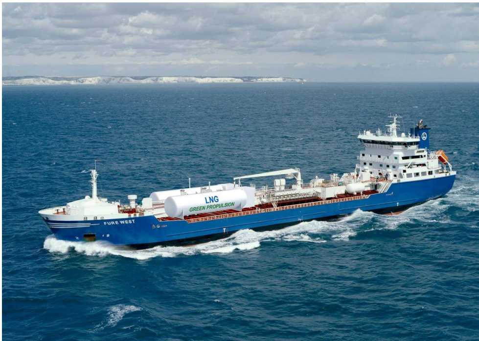
Figure 11 Picture of Fure West with LNG tanks on deck (Furetank 2017)
