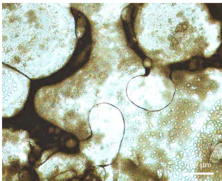
Figure 4.13: Effect of attempt to form Pickering emulsion with TiO 2 nanoparticles.
