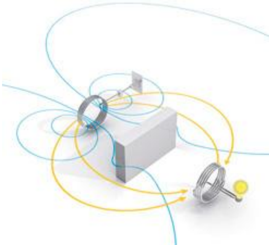
FIGURE 7 THE PRINCIPAL FUNCTION OF WITRICITY, WHERE A MAGNETIC FIELD (BLUE LINES) GENERATED BY THE WITRICITY SOURCE ENABLES ENERGY TRANSFER (YELLOW LINES) AROUND AN OBSTACLE IN ORDER TO POWER A LIGHTBULB CONNECTED TO THE WITRICITY CAPTURE DEVICE.
