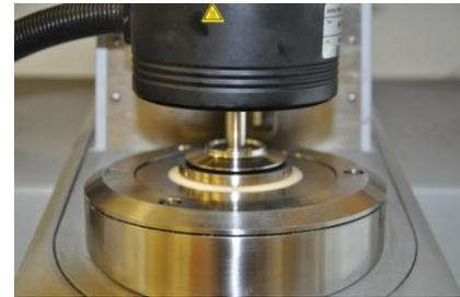
Figure 7c Probe in measuring position
