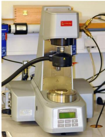
Figure 7a The Physica MCR
