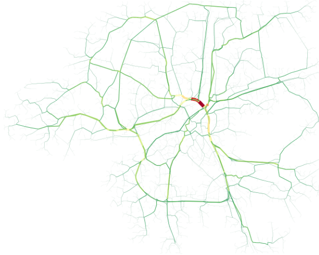
Figure 4.4: The figure shows the resulting betweenness centrality in Gothenburg, where red means a high value. The BC predicts that there will be heavy traffic in Tingstadstunneln. A high flow of traffic does not necessarily lead to congestion.
