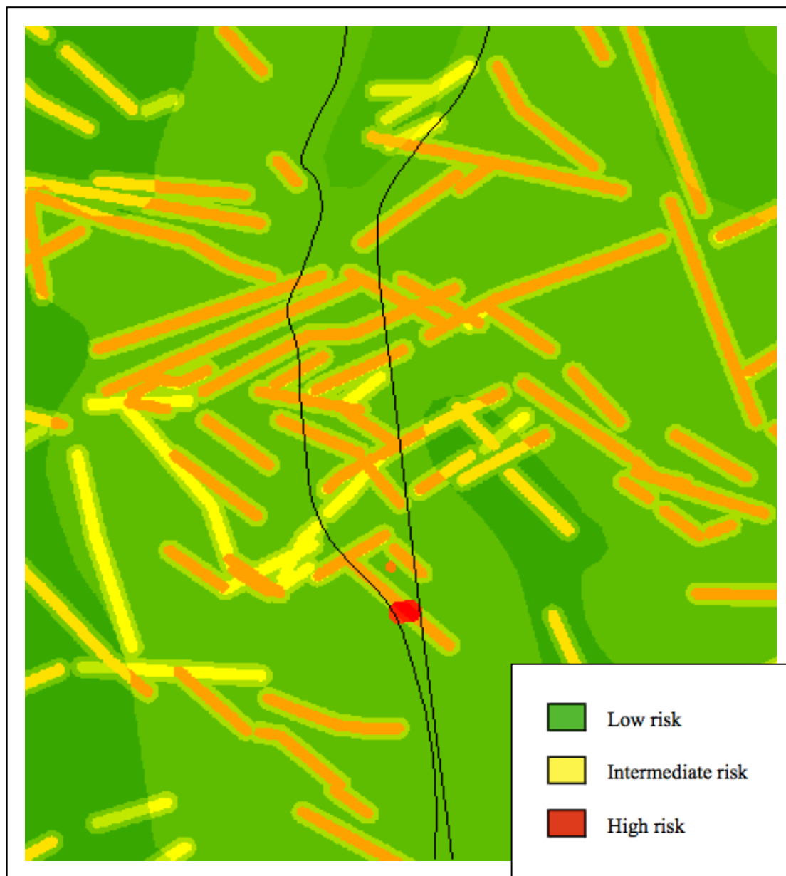
Figure 8.11 Preliminary risk map for the aquifer Omeya golf and residential oasis. The black lines indicate the main road B1 (the right line) and the railway between Windhoek and Rehoboth (the left line). Omeya is situated between the two.
