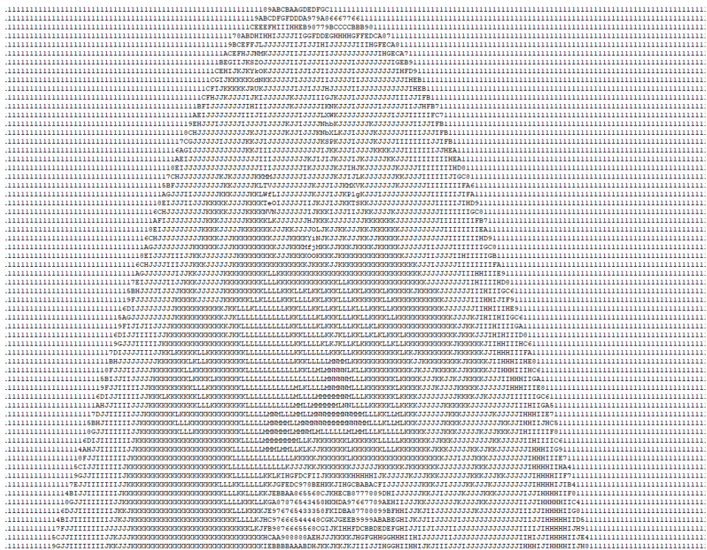
Figure 2.5: A visualization of a head-and-neck-phantom in the format of an eggsphant-file. Each number or letter represent a certain material.
