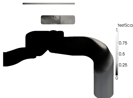
Figure 3.16: The passive scalar is visualised at 360 CAD.
