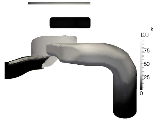
Figure 3.31: The turbulent kinetic energy visualised at 0 CAD using. The k-\omega turbulence model is used.
