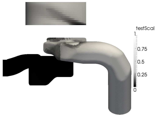
Figure 3.14: The passive scalar is visualised at 285 CAD.
