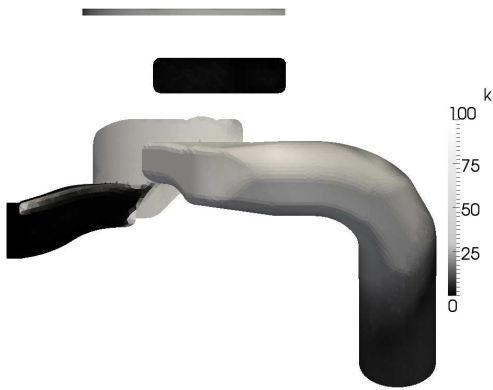
Figure 3.30: The turbulent kinetic energy visualised at 0 CAD using. The k-\varepsilon turbulence model is used.
