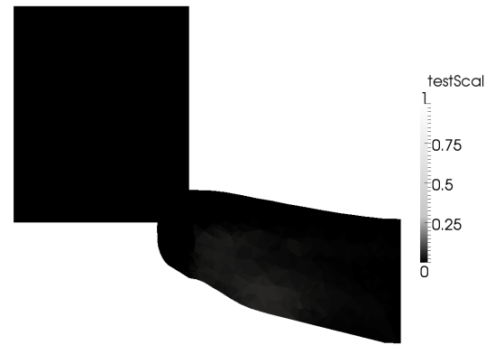
Figure 3.18: The passive scalar visualised in the exhaust channel at 120 CAD.
