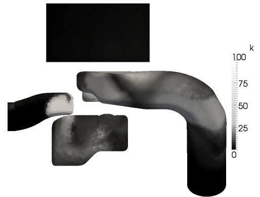
Figure 3.33: The turbulent kinetic energy visualised at 101 CAD using. The k-\omega turbulence model is used.
