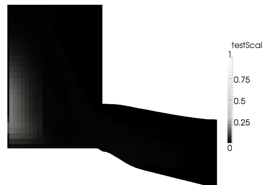
Figure 3.20: The passive scalar visualised in the exhaust channel at 180 CAD.
