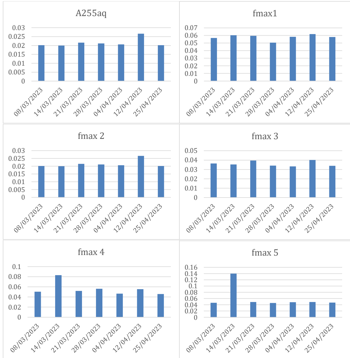
Figure 26. Displaying different fluorescence components in sand filter 2 over the sampling period, and A255aq which is the absorbance.
