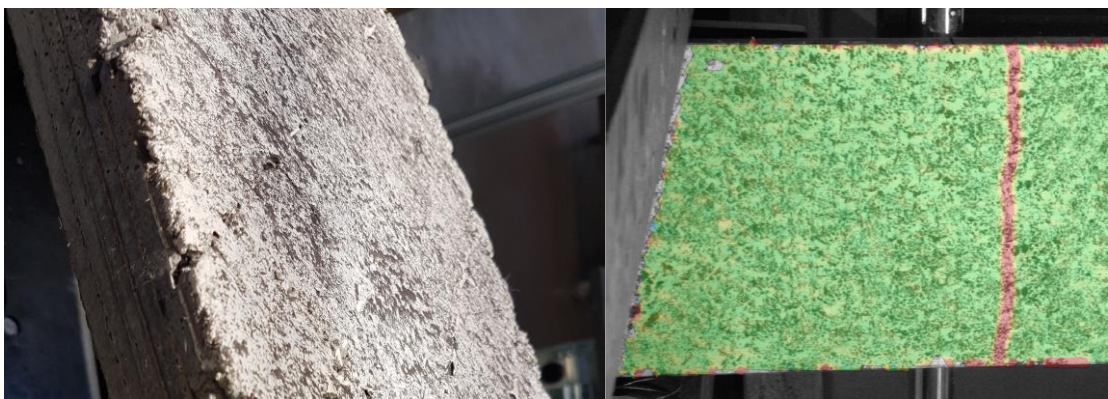
Fig 3.8: Photos of the dotted pattern painted on the specimens.
