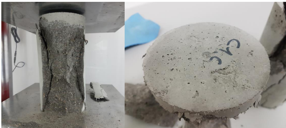
Fig 3.12: Photo of crack pattern from compression test.
