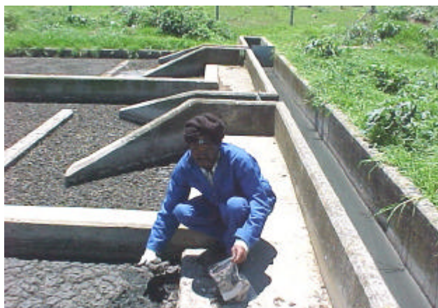
Figure 27 Sludge sampling from drying beds.
