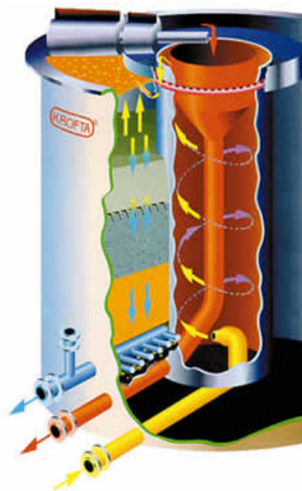
Figure 2. Dissolved-air flotation unit used for thickening waste activated sludge (web ref 1).
