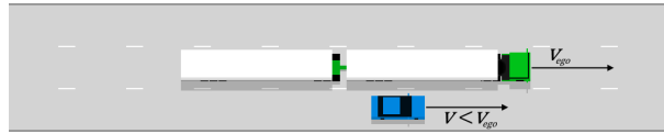
Figure A.6: Scenario 6: Multiple lanes, the ego vehicle attempts to overtake a vehicle in another lane.
