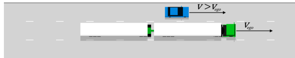
Figure A.8: Scenario 8: Multiple lanes where the ego vehicle is being overtaken by a vehicle in another lane.
