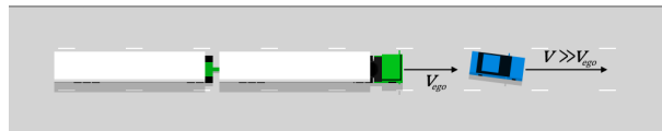
Figure A.9: Scenario 9: Multiple lanes where a vehicle changes into the ego vehicle's lane shortly after overtaking the ego vehicle.
