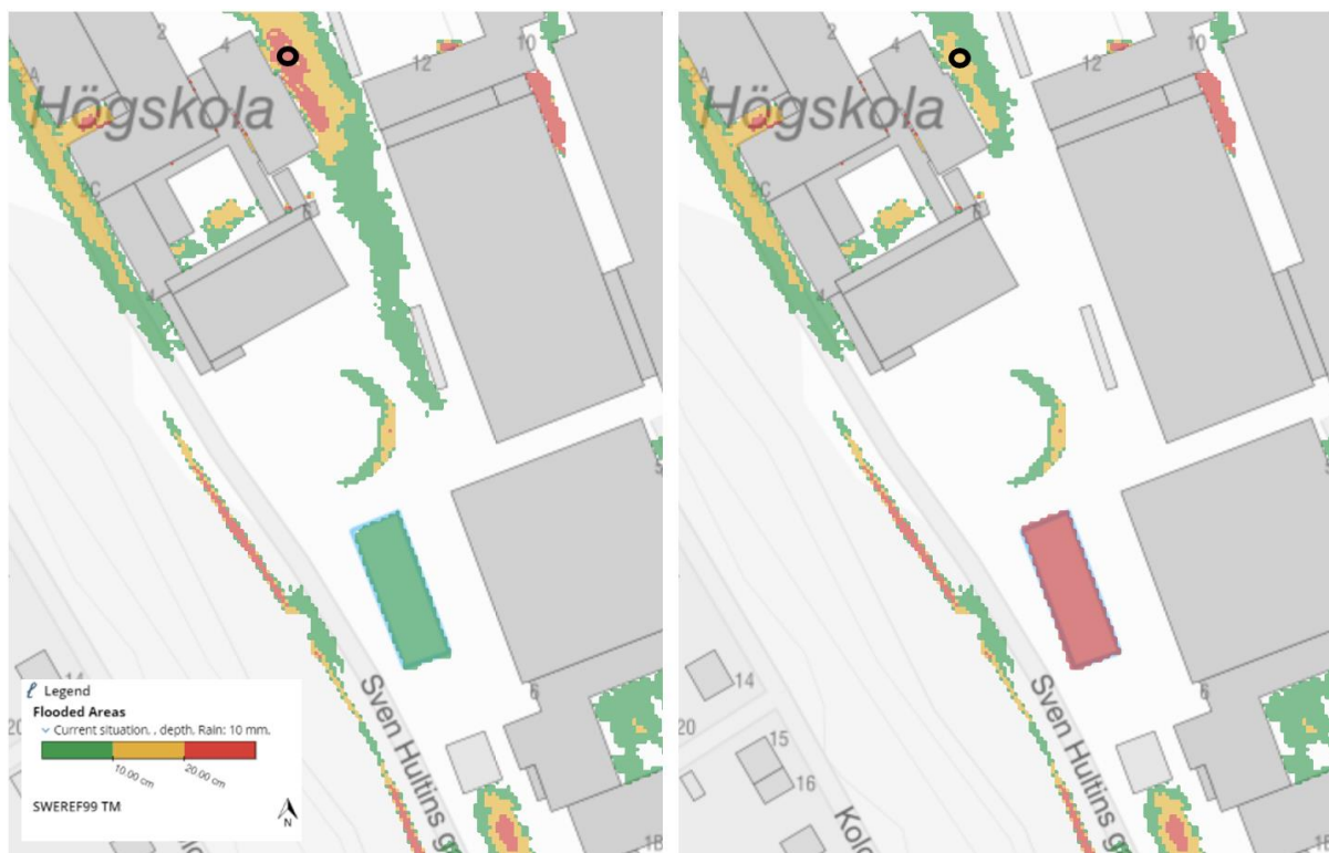
Figure 5.13 Left picture: Without implemented solutions with 10 mm of precipitation. Right picture: With implemented solutions with 10 mm of precipitation. Both simulations from SCALGO Live.
