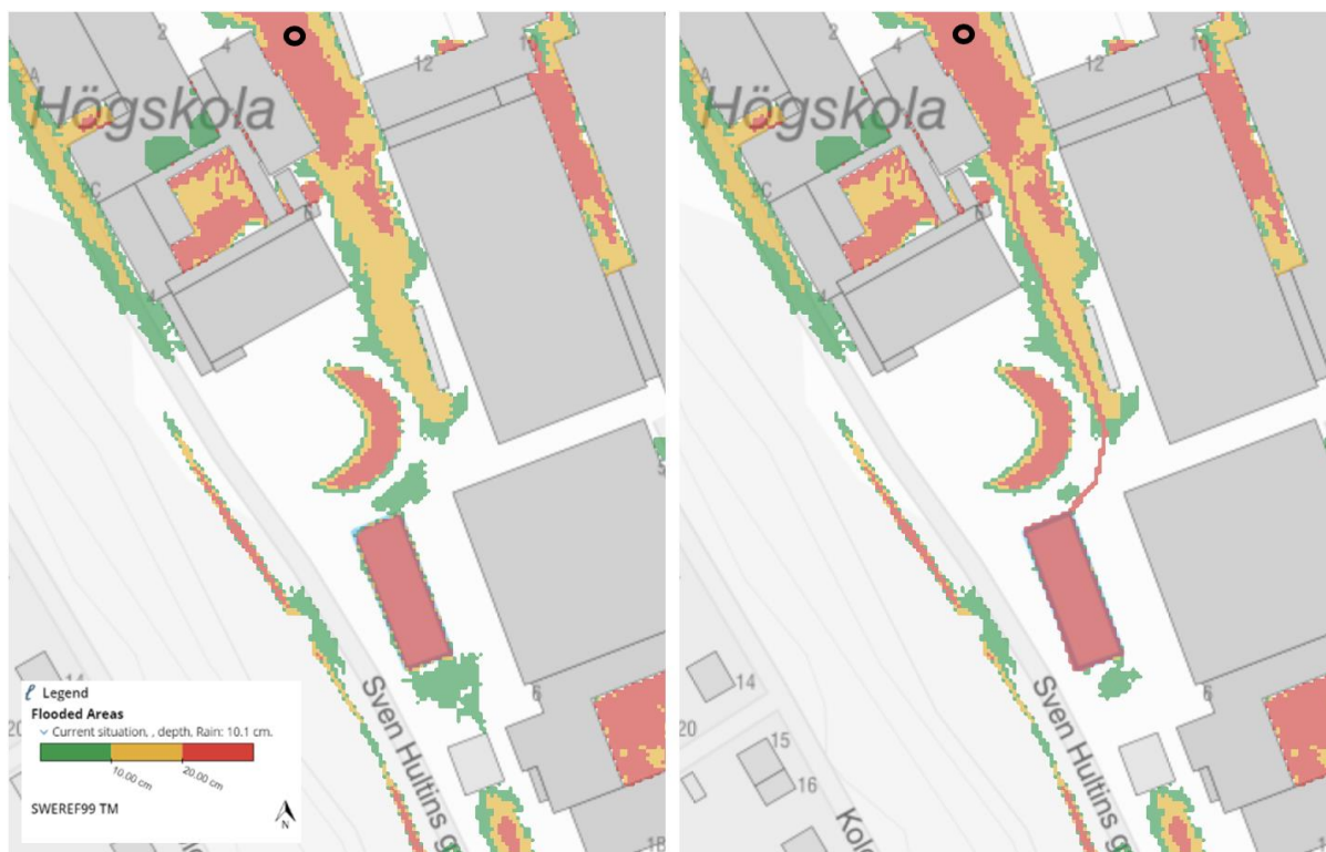
Figure 5.14 Left picture: Without implemented solutions during a cloudburst of 101 mm. Right picture: With implemented solutions during a cloudburst of 101 mm. Both simulations from SCALGO Live.
