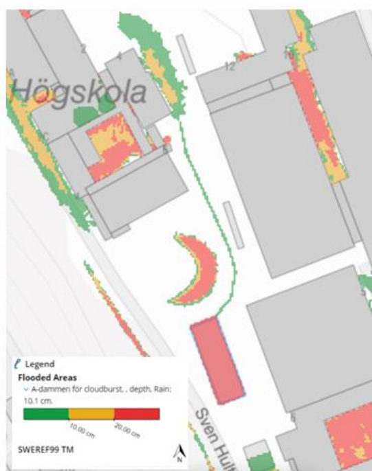
Figure 5.15 A-dammen lowered to a level of +39.23 meters in order to store all of the water from a cloudburst of 101 mm. Simulation from SCALGO Live.
