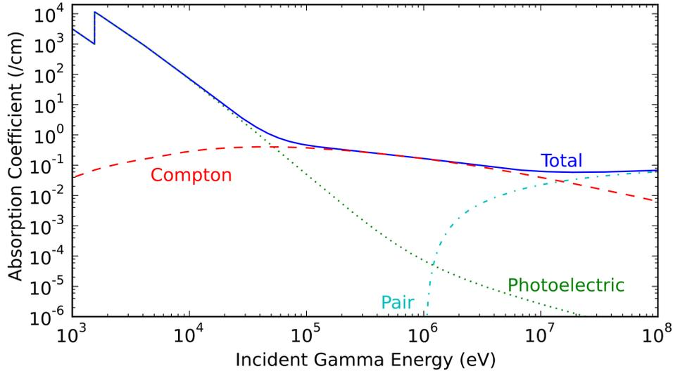
**Figure 1.3:** *The total absorption coefficient and the contribution from the different interaction types as a function of the  $\gamma$  energy. For this example Al has been used. When other materials are used the values change but the general pattern remains. Figure from Ref. [9].*
