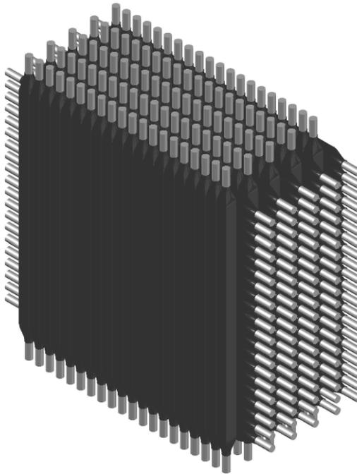
**Figure 1.5:** *A basic model of the LAND-detector. Each paddle is 2 meter long and 10 cm wide. It has 10 planes, each 10 cm thick.*
