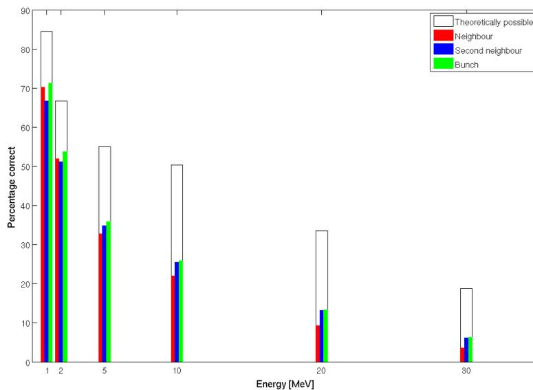
**Figure 2.7:** How often the different adback routines are correct when two protons are shot at random directions in the Crystal Ball for different energies. The result for 300 MeV protons are not visible because the protons are not stopped in the crystal, thus is not the entire energy deposited in the Crystal Ball.
