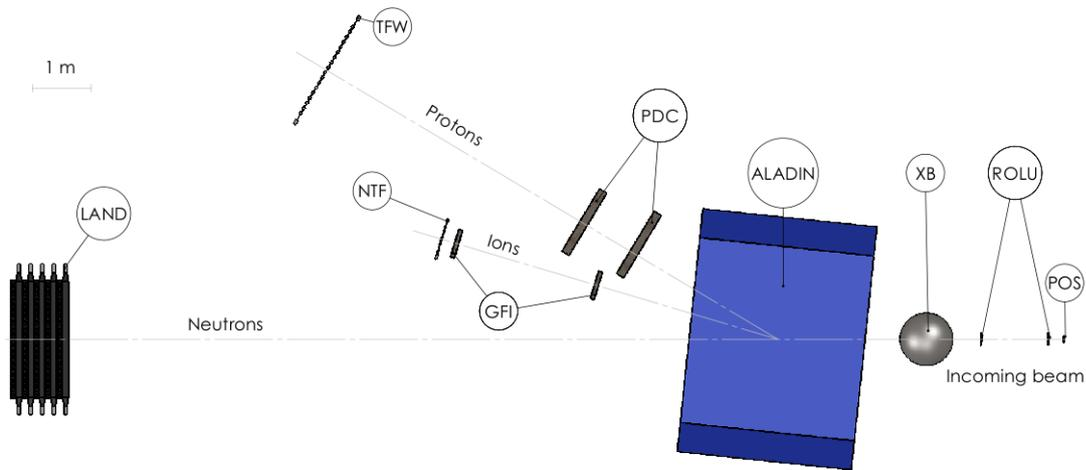
**Figure 1.1:** A sketch of the LAND-setup as seen from above. The target is placed inside the Crystal Ball (XB).
