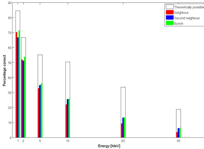
**Figure 2.6:** How often the different adback routines are correct when two gamma-particles are shot at random directions in the Crystal Ball for different energies.
