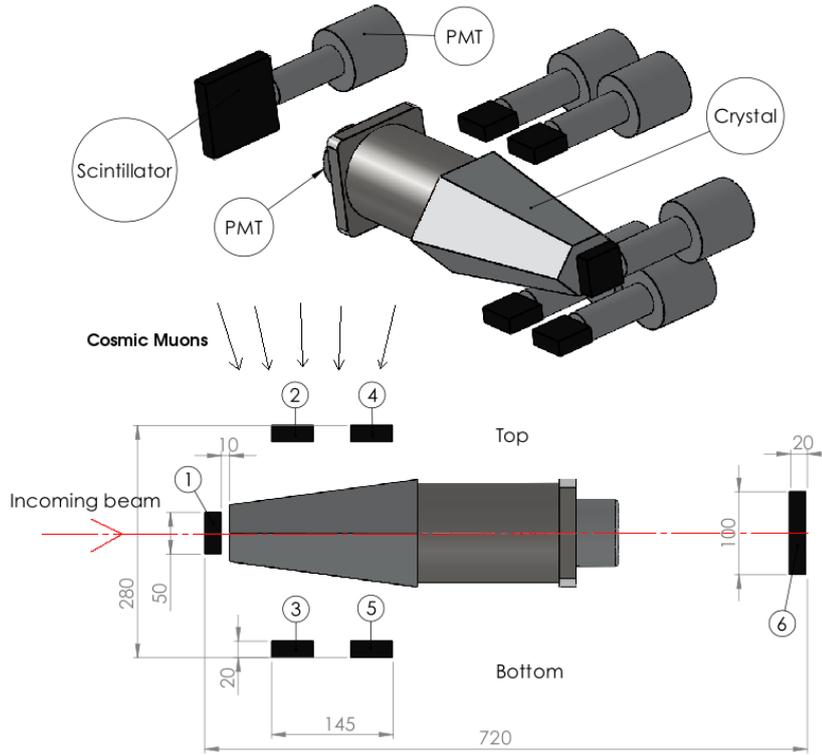
**Figure 4.2:** A schematic drawing of the CXB detection system. The numbers in the lower drawing indicate the numbering of the scintillators used during the experiment. Scintillator 1 is in front and scintillator 6 in the back. All dimensions are given in mm.
