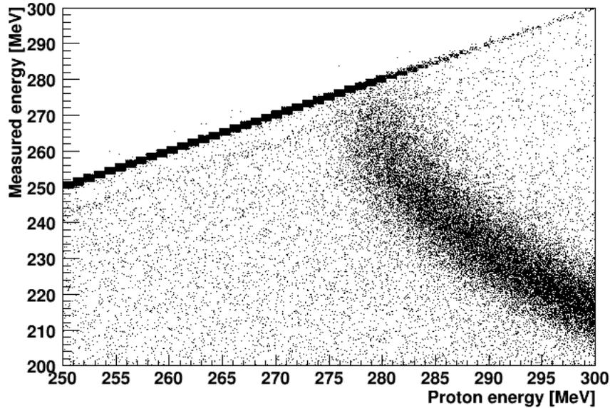
**Figure 2.3:** *The energy deposited in the Crystal Ball in each event plotted against the energy of the incident proton. The punch-through energy is seen at about 280 MeV. The punch-through limit is rather distinct even though some protons are completely stopped also beyond the limit.*
