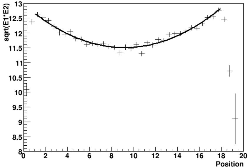
**Figure 3.1:** The plot shows  $\sqrt{E_1 E_2}$  in uncalibrated units versus the position of the hit expressed in paddles. The black line is a second degree polynomial fit. The data used were obtained during experiment S245 for paddle No. 12 in plane No. 5 of the LAND detector.
