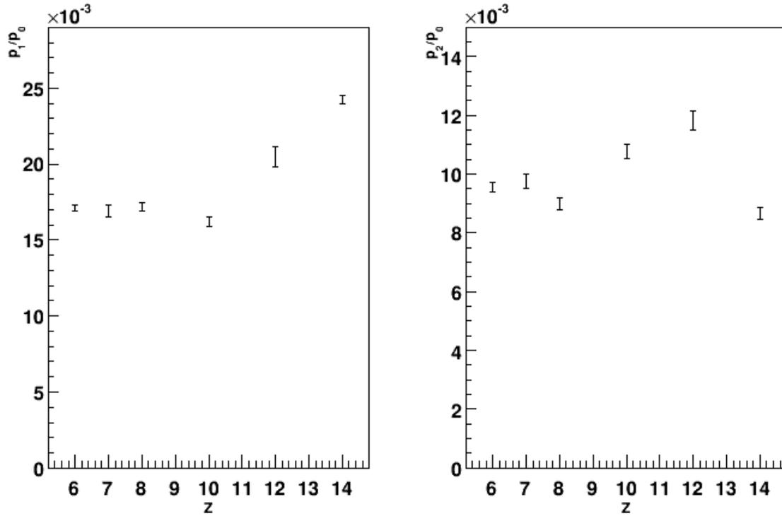
**Figure 3.7:** The coefficients  $\frac{p_1}{p_0}$  and  $\frac{p_2}{p_0}$  for different ions. As can be seen, both  $\frac{p_1}{p_0}$  and  $\frac{p_2}{p_0}$  are almost the same for different  $z$ .
