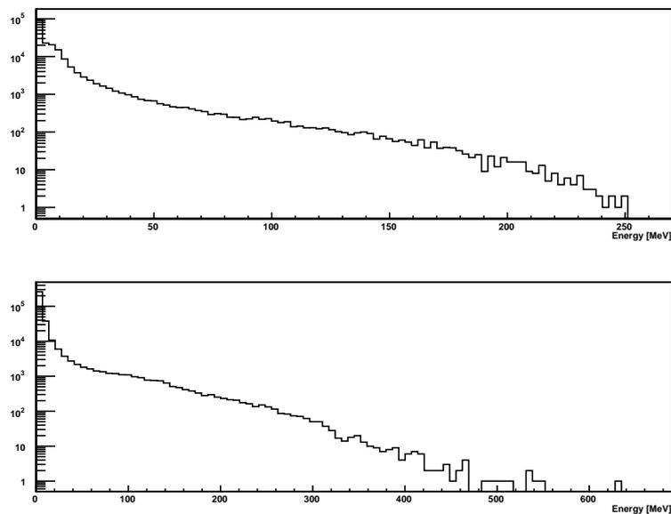
**Figure 2.4:** *The energy deposited in crystals by 250 MeV neutrons (upper) and 300 MeV neutrons (lower). The extra energy appearing in the lower histogram is suspected to originate from problems in the simulations.*
