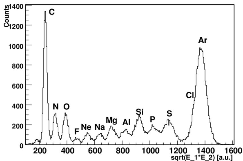
**Figure 3.4:** *The energy spectrum for paddle No. 4 in the y-plane at the intersection with paddle No. 3 in the x-plane. Each peak correspond to one ion species. Data taken from experiment S327.*
