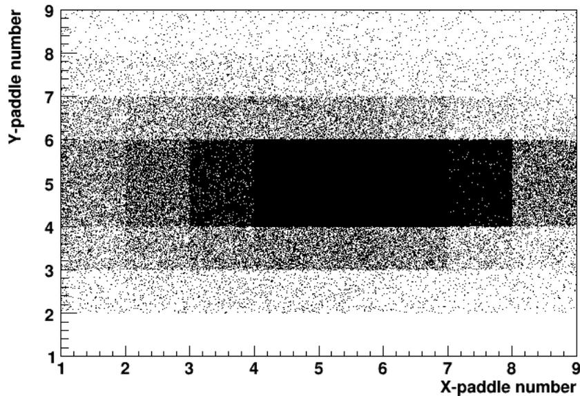
**Figure 3.3:** *The hit pattern for the NTF from experiment S327. A dot between 2 and 3 correspond to a hit somewhere in paddle No. 2, a dot between 3 and 4 correspond to a hit somewhere in paddle No. 3 and so on. Paddle No. 1 in the y-plane did not work properly during the experiment.*
