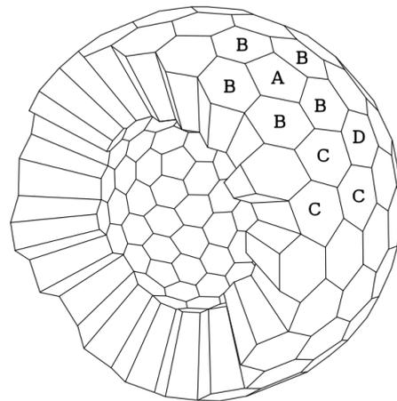
**Figure 1.2:** A schematic view of the crystals building up the crystal ball. The letters mark the shape of the crystal. Figure from Ref. [6].
