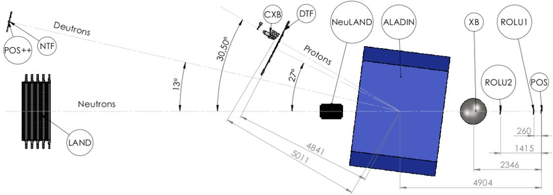
**Figure 4.1:** *The experimental setup during experiment S406. Not all the detectors present in the experiment are shown, but the most important ones for the experiment and for the CXB. All distances are given in mm.*
