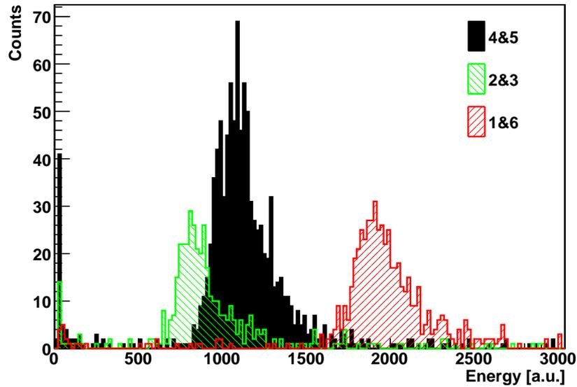
**Figure 4.4:** *The energy deposited in the crystal by cosmic muons with different path lengths through the crystal. The legend tells which scintillator pairs have coincident hits for each colour.*
