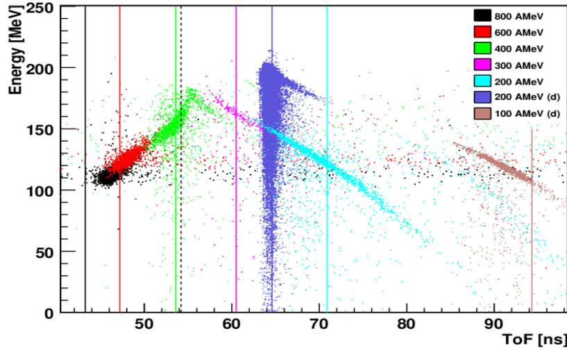
**Figure 4.5:** The energy deposited by protons/deuterons in the CXB crystal plotted against time of flight from the start detector (POS) to the CXB. Vertical lines mark the expected time of flight for the related run and the dashed line is the expected time of flight for the punch-through limit. The two runs marked with (d) in the legend are sweep runs with deuterons. The 200 A MeV deuteron sweep run has been used for offset calibration, using the energy value derived from the magnet current.
