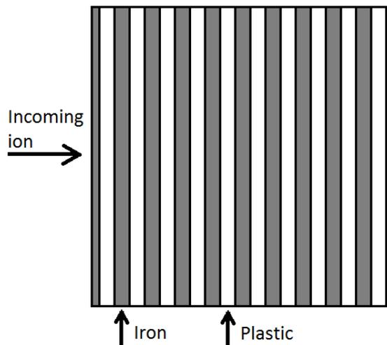
**Figure 1.4:** A cross-sectional view of a paddle used in the LAND detector. The first and last iron sheets are 2.5 mm thick while the rest are 5 mm.
