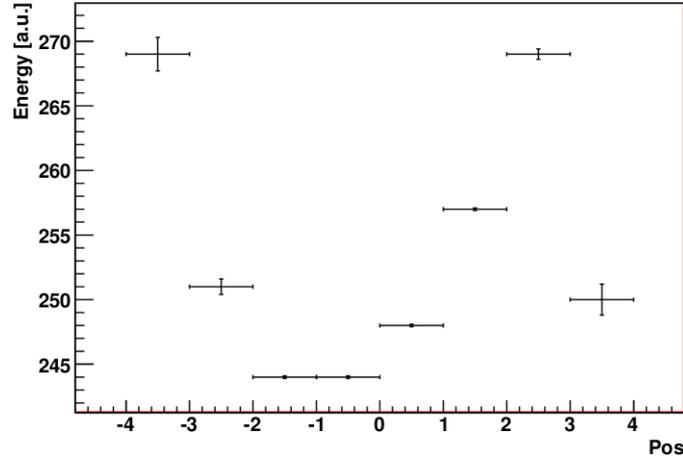
**Figure 3.6:** *The energy in paddle No. 4 of the y-plane in the NTF-detector plotted against the hit position in the paddle, i.e. what intersection the ion passed. For this plot the carbon ions have been used.*
