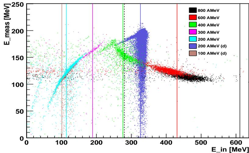
**Figure 4.6:** The measured energy versus the incoming kinetic energy calculated from the time of flight, see Fig. 4.5 and corrected for the energy loss in the plastic scintillators, see text. The vertical lines are the expected energy in that run and the dashed line is the expected punch-through energy.
