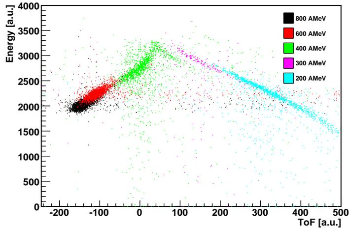
**Figure 4.3:** *The energy deposited in the crystal as a function of the time of flight of the protons between the POS and CXB detectors. The different colours correspond to different beam energy settings. Both axes are uncalibrated.*
