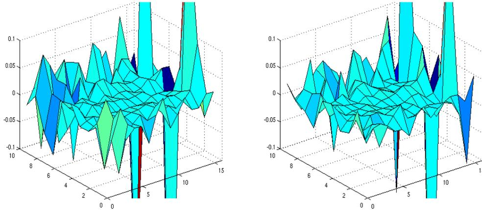
**Figure A.5:** *The energy difference at each paddle intersection in the TFW given from the script `phase1` during experiment `s327`. The left figure is the original difference and the right figure shows the difference after the correction.*
