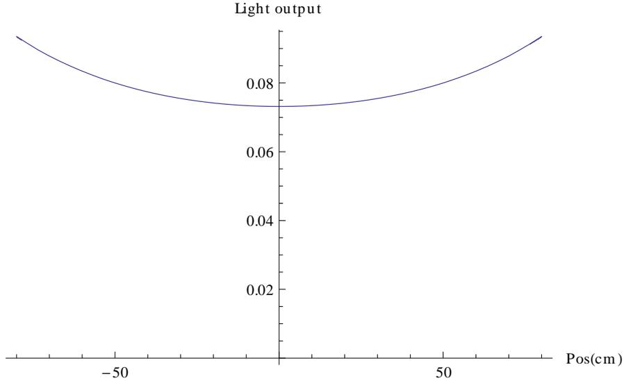
**Figure 3.2:** The function  $\sqrt{E_1 E_2}$  for a LAND scintillator bar when using values  $f(\lambda) \approx 180$  cm,  $\gamma = 58^\circ$ ,  $\rho = 0.985$  and  $\alpha = 0.25$ .
