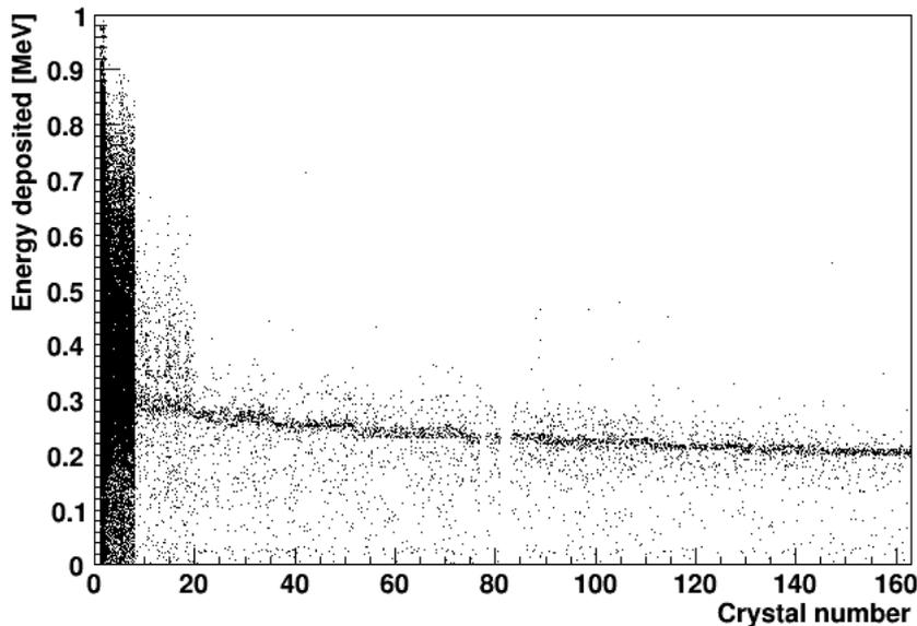
**Figure 2.2:** *The energy distribution for the crystals when shooting 1 MeV  $\gamma$ -rays in the middle of crystal No. 1. Crystal No. 2–7 are neighbours of crystal No. 1 and No. 8–19 are second neighbours, i.e. neighbours to the neighbours.*
