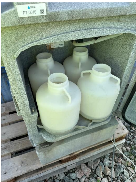
Figure 10. Automatic ISCO sampler (Photo by F. Hadi).
