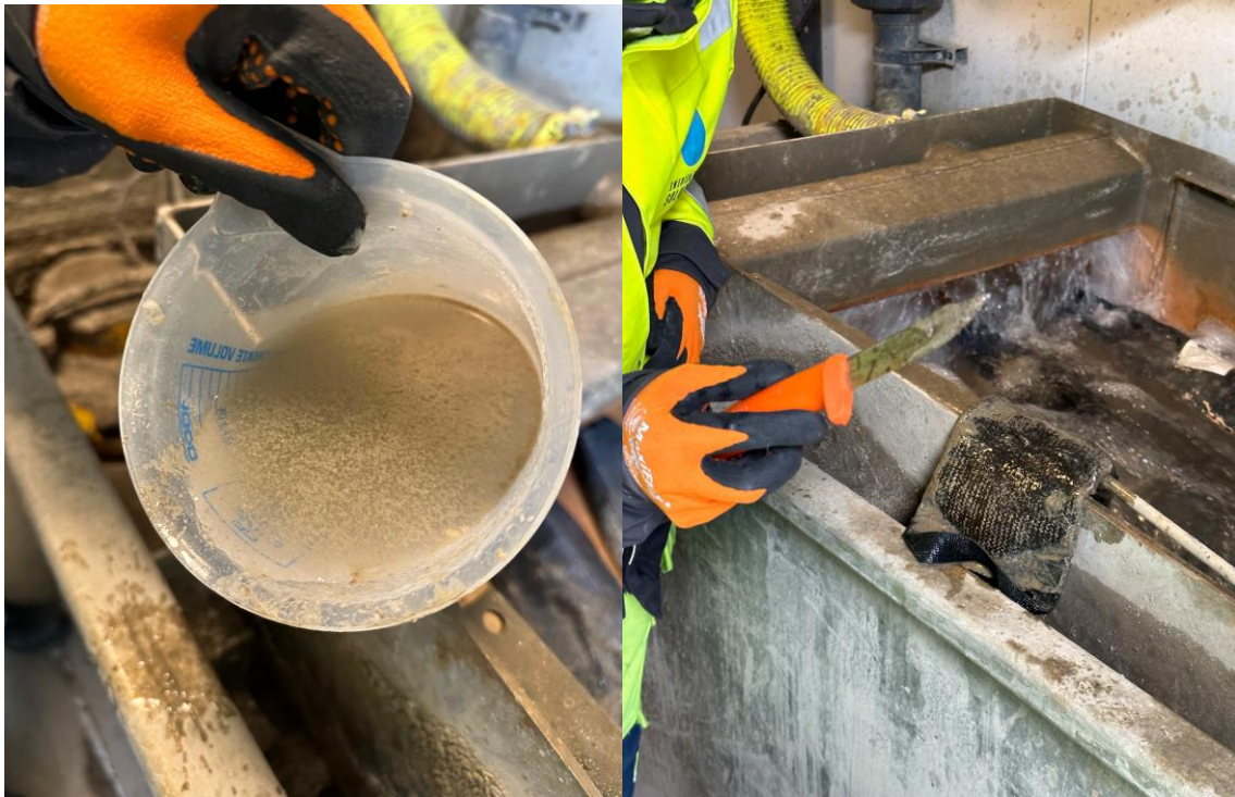
Figure 6. Chitosan flocculation with excess water from building sites. The beaker has been dosed with chitosan to start the flocculation process (Photo by A. Nuur).
