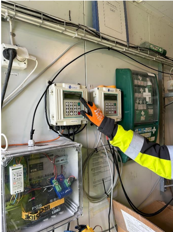
Figure 9. Measuring board for automated assessment of turbidity, conductivity, pH, and flow rate (Photo by F. Hadi).
