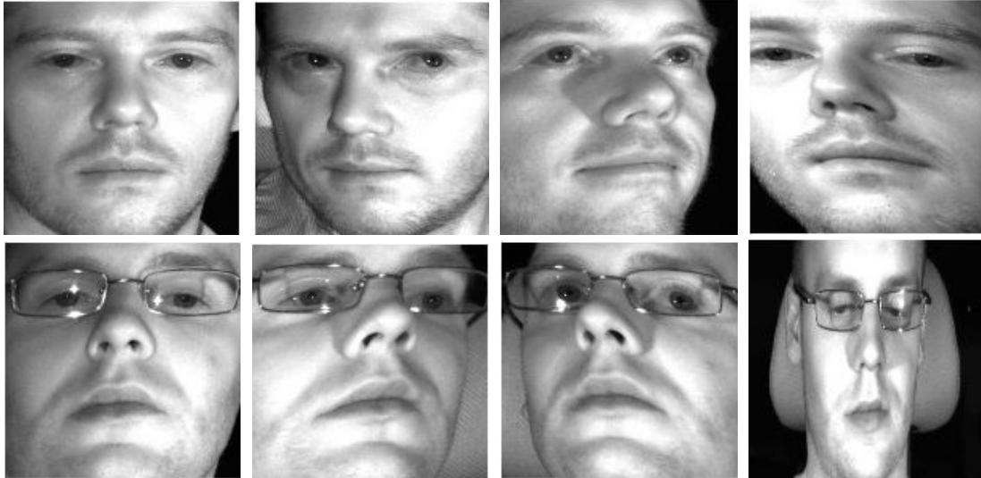
Figure 5.1: A set of aligned faces. The cropping is worse for faces rotated around the cameras y -axis, because the affine transformation assumes that the face is full frontal. The right-most column contains two cases where the feature detector has provided faulty feature points, yielding a badly aligned or cropped image.
