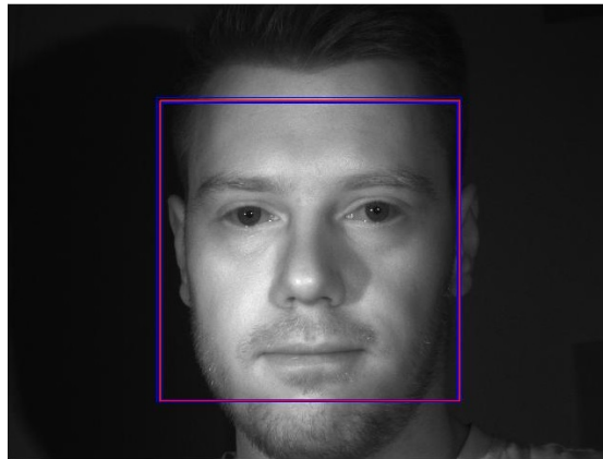
Figure 4.4: A face detected using the Viola-Jones algorithm and OpenCV Haar-cascades. The blue boxes represent individual detections made by different Haar-cascades, whereas the red box is the mean box of all detections and the final output of the detector.
