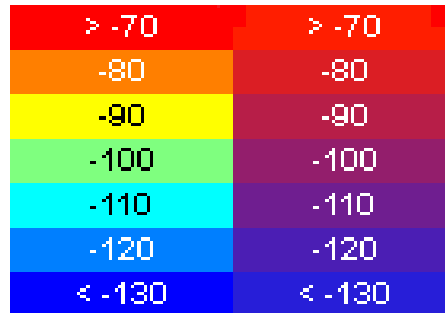
Figure 5.5: RSSI legends compared with the two scales
