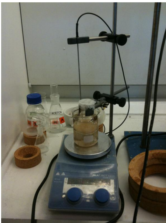
Picture 2. The setup for the sulfonation.
