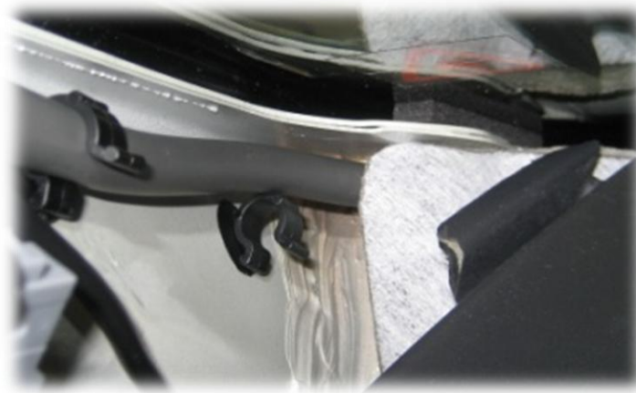
Figure 3.5 – Illustration of new higher clip position
