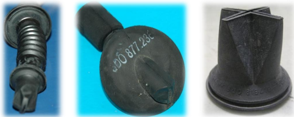
Figure 4.3 – Pictures of competitors different drain plugs. Left - Volkswagen Eos. Centre - Volkswagen Phaeton. Right - Audi A4
