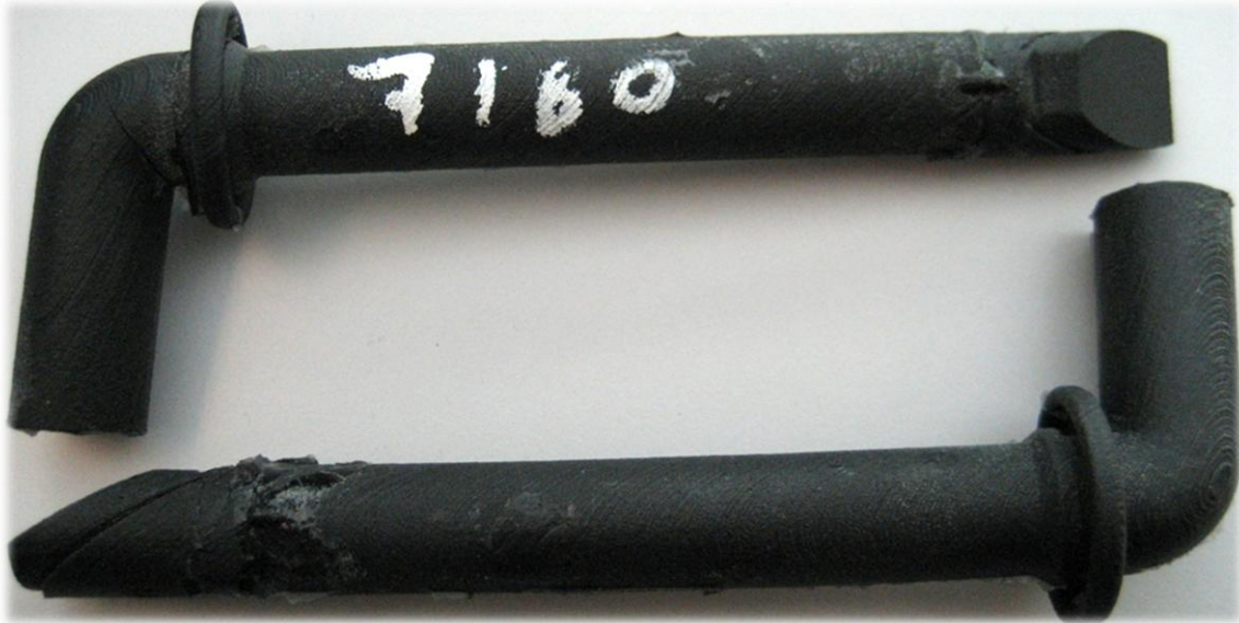
Figure 5.15 - Picture of two different drain plug prototypes. The upper one is with lid facing upwards while the lower one has its lid facing the side.
