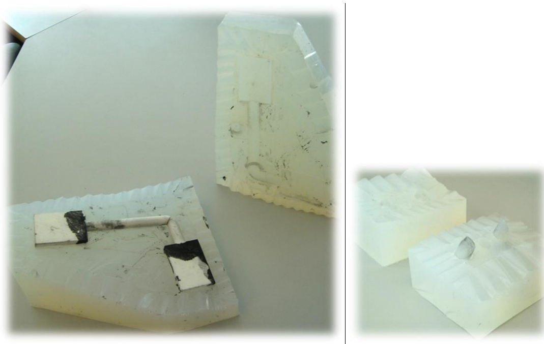
Figure 5.14 - Picture of the silicone tool. Left: Main part of the drain plug, split in two parts, with the two inner core parts mounted. Right: Tool for the non-return valve
