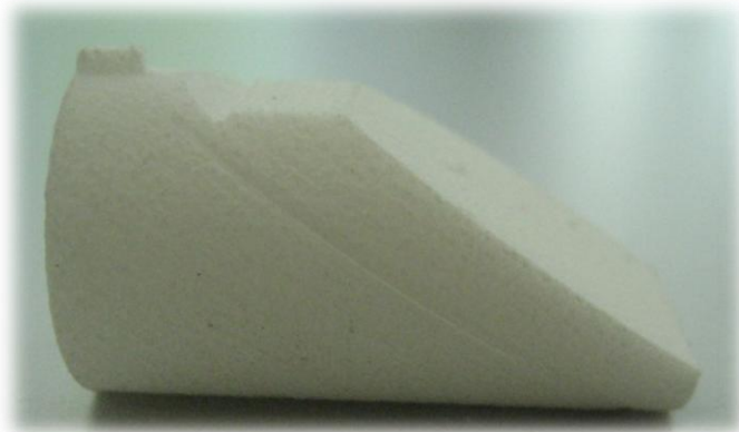
Figure 5.13 - Picture showing FFF core of the drain plug non-return valve
