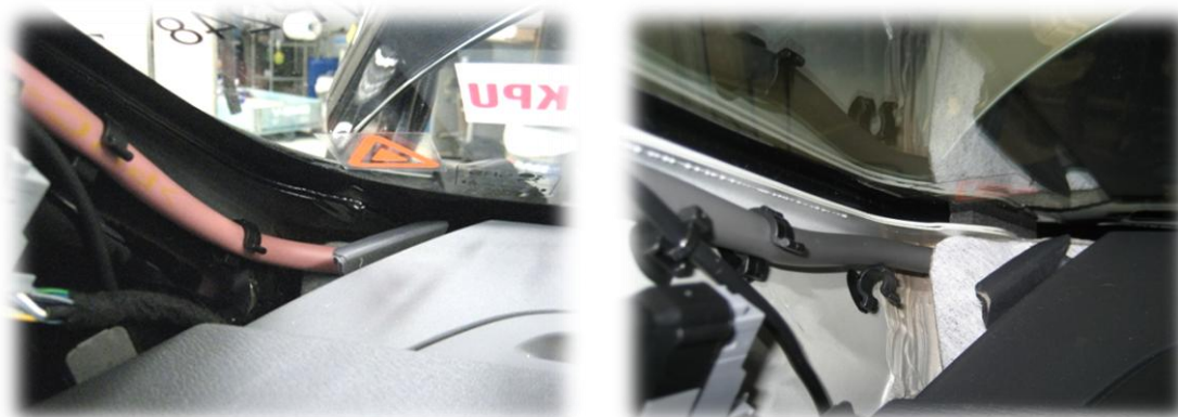
Figure 4.14 - Pictures of different drain hose positions. Left - Original position. Right - Modified position
