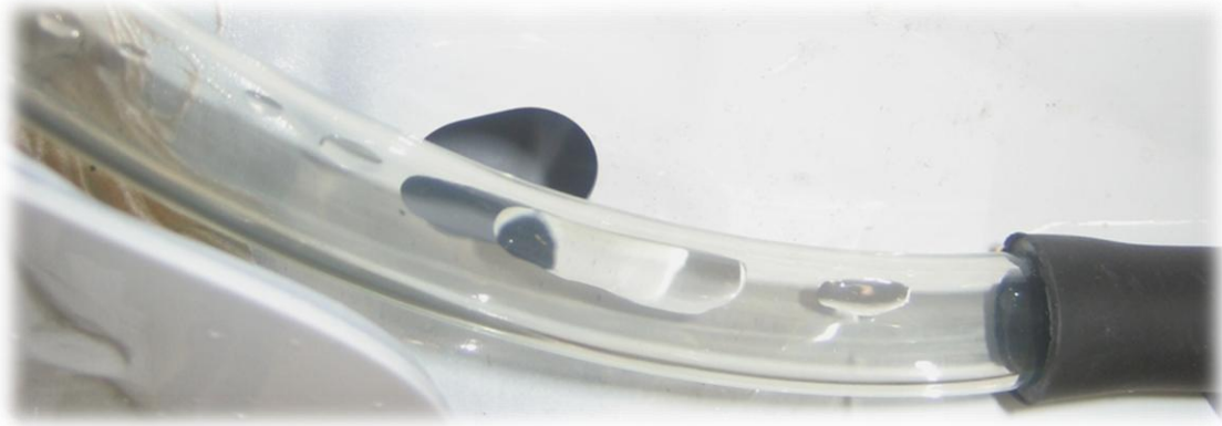
Figure 4.13 - Lower water trap with larger water piles
