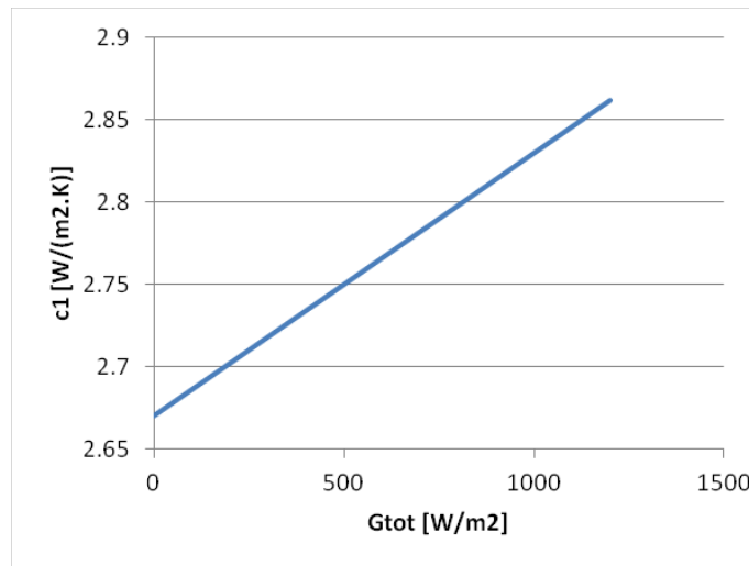
Figure 4.9 Illustration of c_1 's dependency on total solar irradiance for a flat plate collector using the Birr estimation
