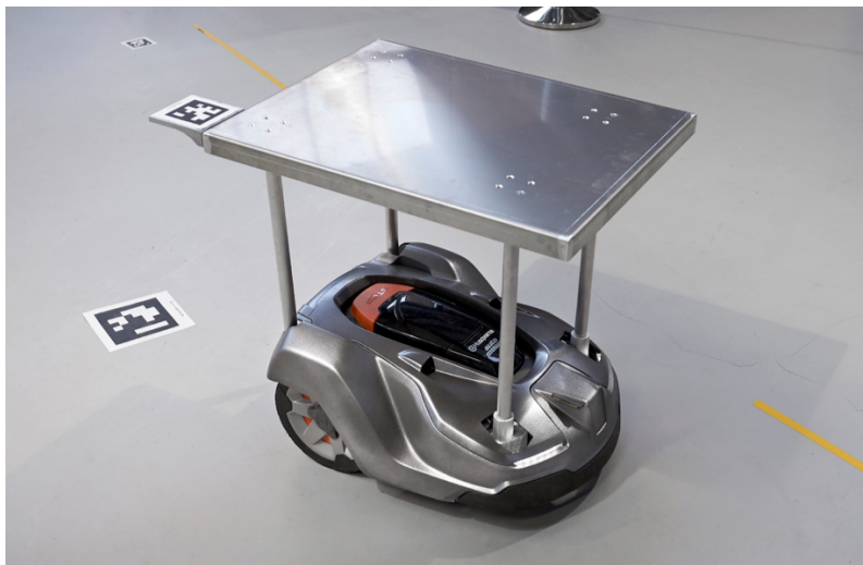
Figure 2.2: A prototype of Volvo Truck’s ATR, which is based on a robotic lawnmower from Husqvarna modified with a table and AprilTag. From [1]. Reproduced with permission.
