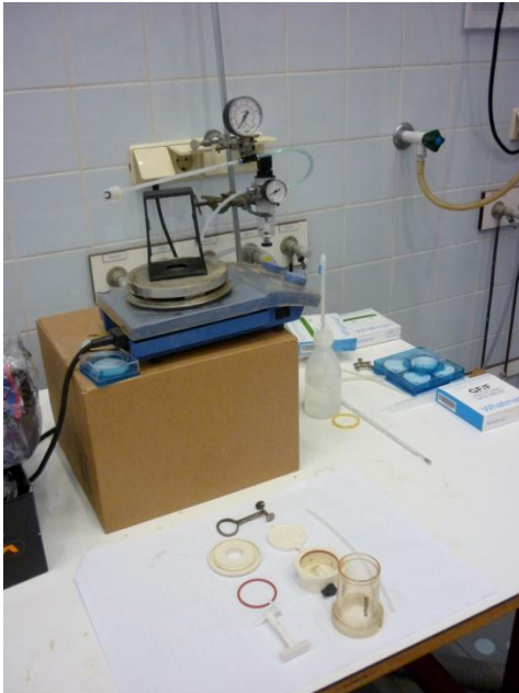
Figure 6 Amicon cell components, stand, magnetic stirrer, pressure valve and 0.22µm filters
