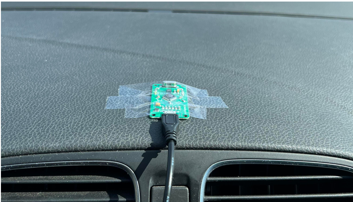
Figure 4.6: How the sensor was attached to a car for data collection.
