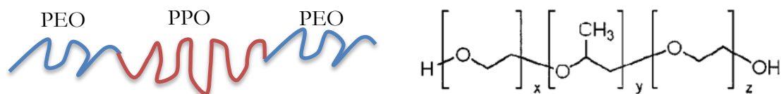
Fig 2.2: The chemical structure of an amphiphilic triblock co-polymer (Trade name Pluronic) used in the present study showing hydrophilic polyethylene oxide (PEO) chains in blue and hydrophobic polypropylene oxide (PPO) chains in red.[21, 33]
