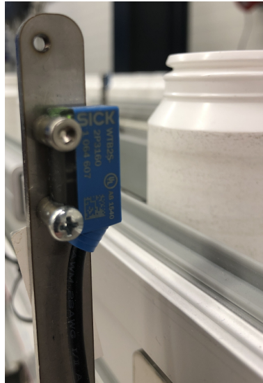
Figure 4.3: The diffuse reflective sensors used on the test rig
