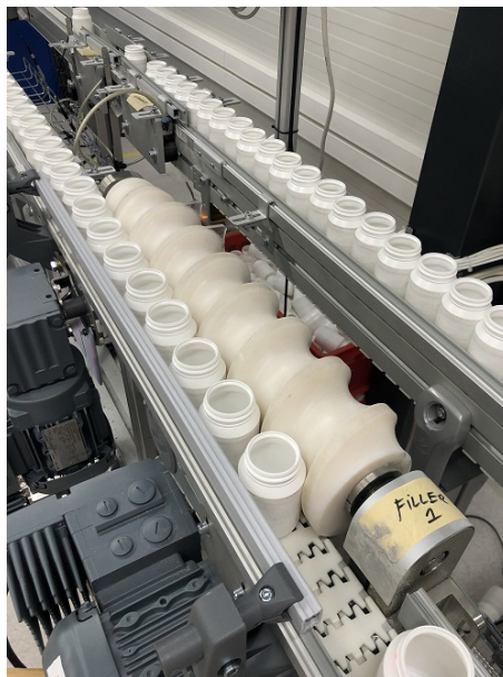
Figure 4.4: One of the motorised screws which is used to mimic a machine
