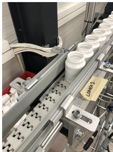
Figure 4.2: The pneumatic air stop which controls the in-feed of the system
