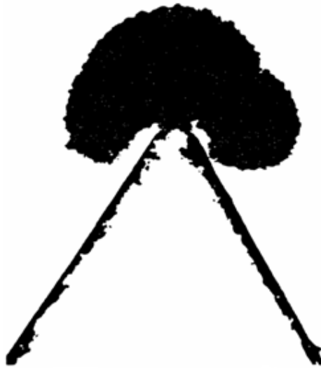
Figure 2.4: Typical shaped vented water tree according to the international standard ASTM D6097 [2].
