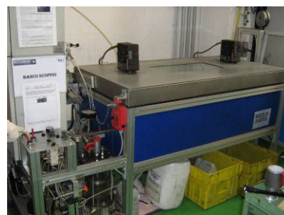
Figure 53 – Hutchinson burst test bench
