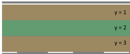
Figure 3.1: Discretization of the lateral position relative to the lane into k = 3 intervals. For instance a car with no lateral offset will have a lane position y = 2 . The intervals have an equal size which it depends on the width of the lane.
