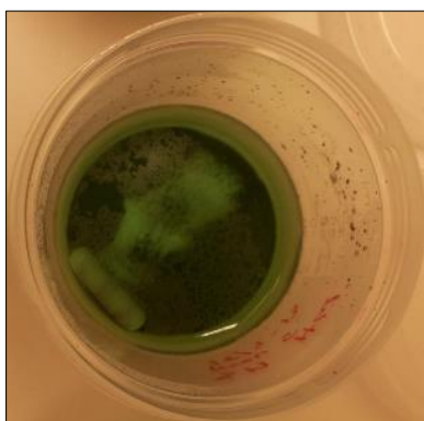
Figure 9: After 94 h of leaching with 3 M HCl solution, a photo was taken of a solution. The black color, present in the bottom of the vessel, is undissolved starting material. This image was representative to the other solutions of 1 and 6 M HCl.
