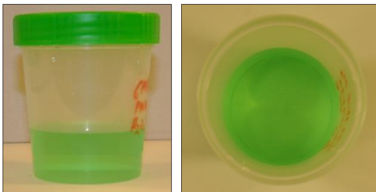
Figure 71: A typical solution (initially 6 M HCl) after it has leached the material during addition of \text{H}_2\text{O}_2 at 75^\circ\text{C} . The solution is very transparent. The solution is viewed from the side (left picture) and from above (right picture).
