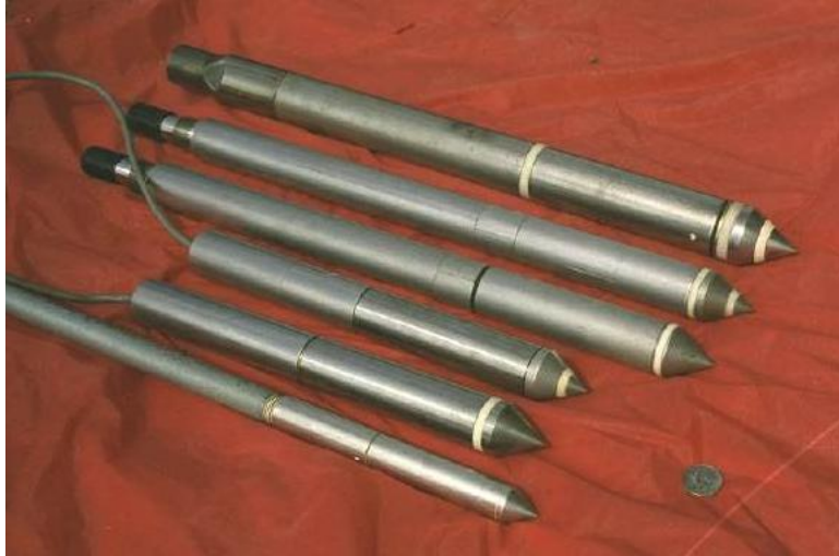
Figure 4 A type of CPT probe (School of Civil & Environmental Engineering).
