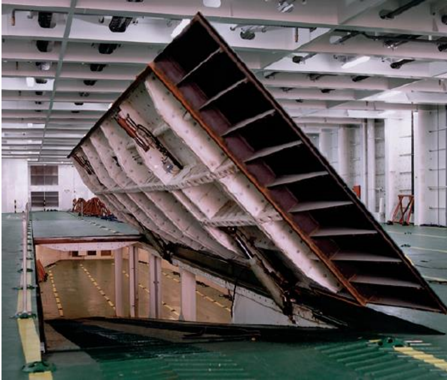
Figure 1.2: Side hinged ramp cover operated by two hydraulic cylinders
