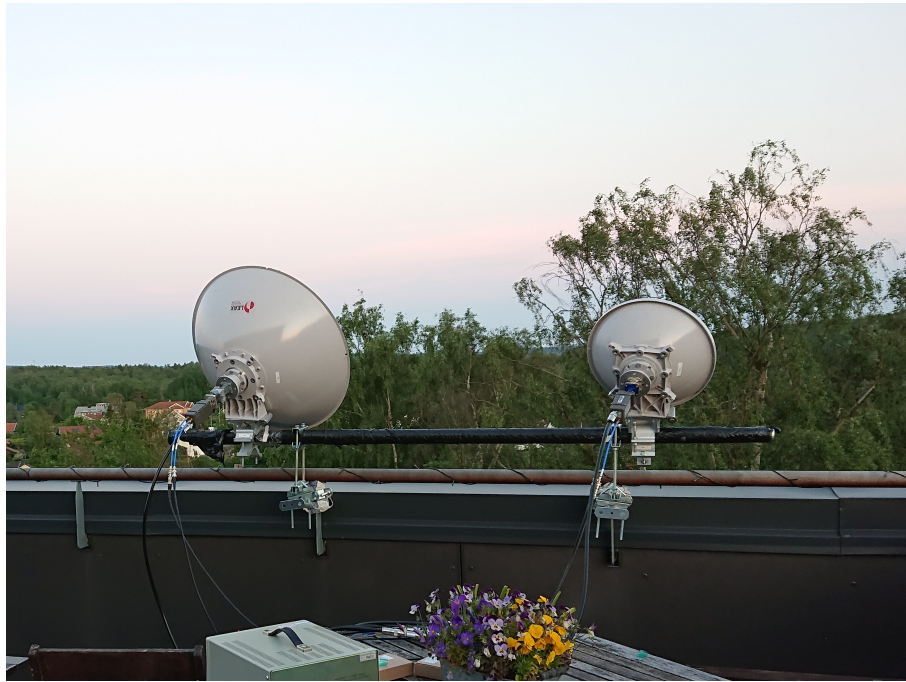
Figure 4.22: The balcony expedition zero-delay verification test antenna setup. Both antennas are aimed directly at the GEO TV-DBS Astra 4A. Special thanks to Vanessa and Per for letting us borrow their apartment and especially spacious balcony for experiments during the day of their wedding.
