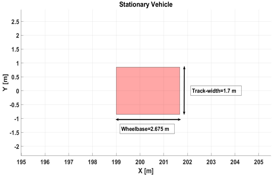
Figure 3.5: Stationary vehicle as an obstacle with dimensions
