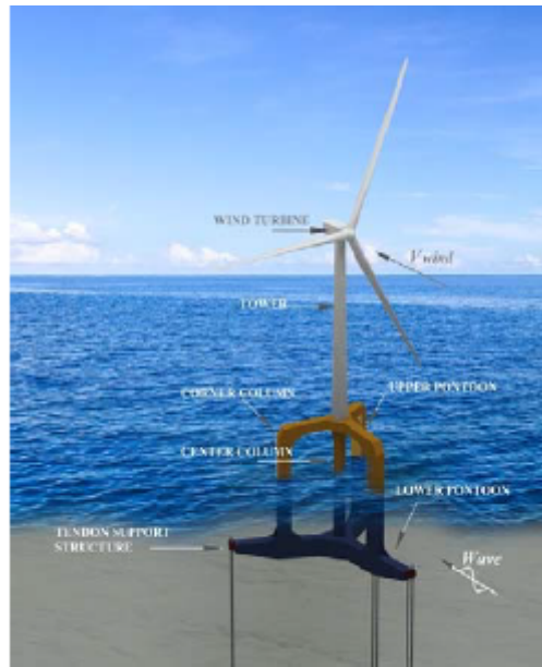
Figure 3.1: Windstar TLP system [49]
