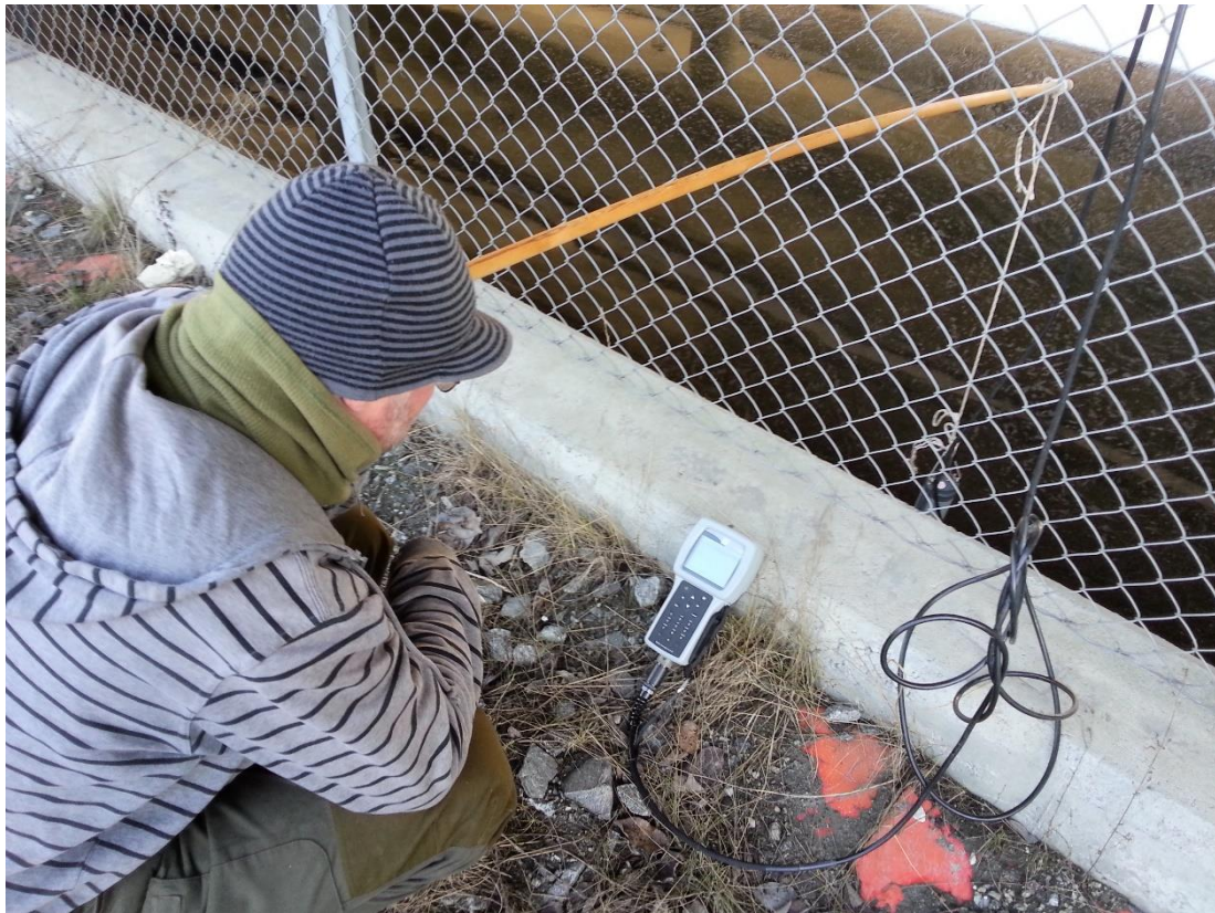
Figure 3. Picture of the water quality sampling with a multi-parameter water quality sonde.
