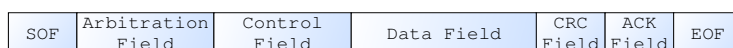
Figure 6 A CAN data frame consist of seven fields. The data field holds the useful information while the other fields only are used during communication.
