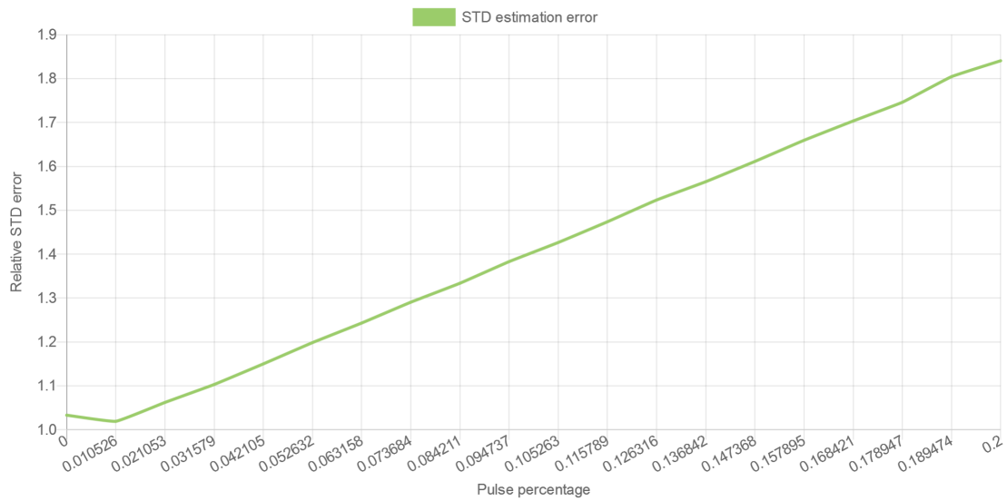
Figure 4.3: Relative STD error as a function of pulse percentage. Data is averaged over 100 traces. The pulses was generated with function 4.1 with a = 160 and c = 7 , the noise had a STD of ten.
