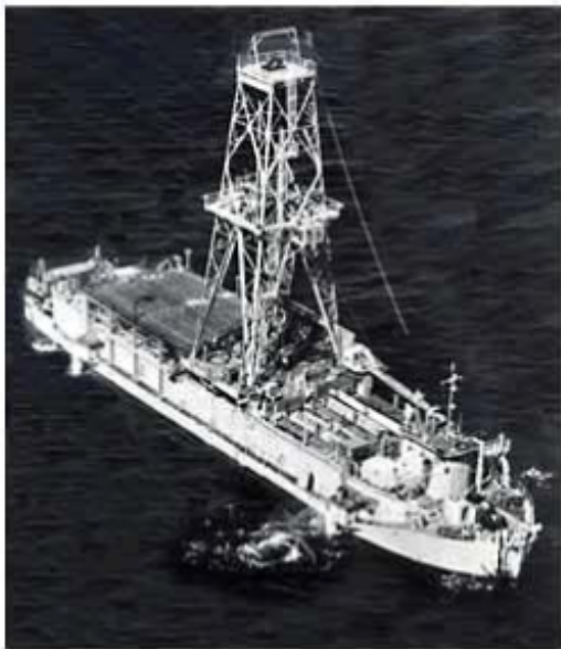
Figure 1.3: The first floater to utilize DP was Cuss 1 in 1961, where it was able to be stationed over a depth of approximately 3500 m and drilled over 180 m beneath the sea floor (NSF photograph).
