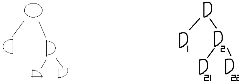
(a) A schematic view over the domain after each branch (b) The union of the branches on each level equals their parents, D_1 \cup D_2 = D , D_{21} \cup D_{22} = D_2 .
