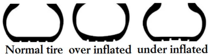
Figure 8: Effect of different Inflation levels on tire figure borrowed from [16].
