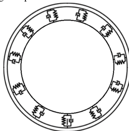
Figure 10: Wheel bearing spring-damper model
