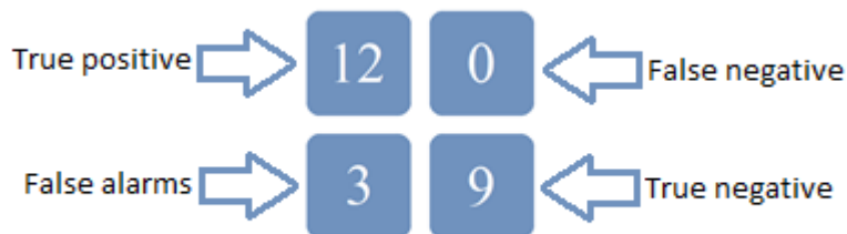
Figure 20: Contingency matrix of the mixed data clustering result
