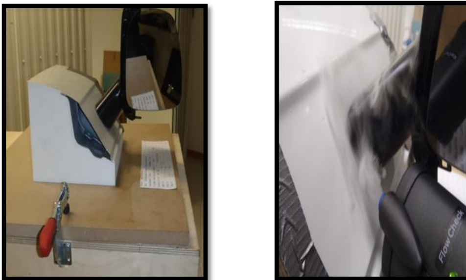
Figure 16 Compressed air test along with smoke gun on side mirror
