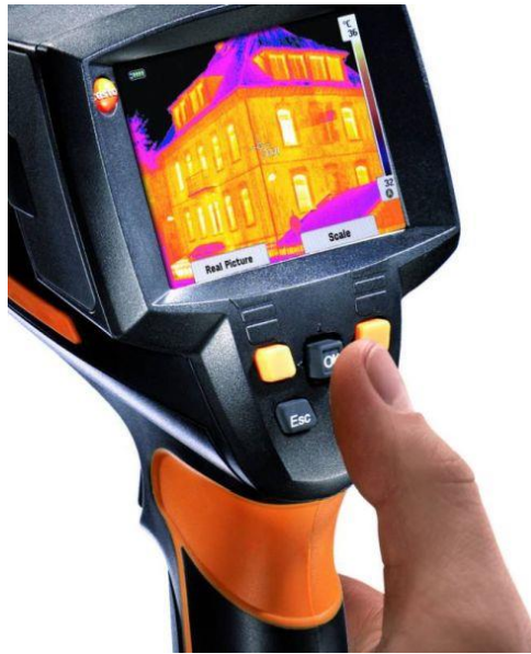
Figure 12 Thermal image camera
