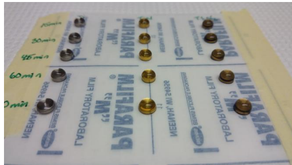
Figure 12. Image shows coins which are being prepared for staining with phalloidin. Three rows with the three different sample groups are seen. From left: Ti, TiN and TiN 2 . On top of each coin is a droplet of block solution.
