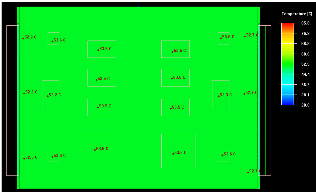
Figure 20 the temperature on the Al-back plate for the TSO card when the vapour chamber is implemented.
