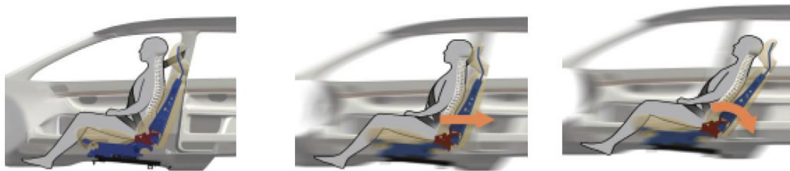
Figure 2 Whiplash Protection System (WHIPS). Normal position → Translational motion → Reclining motion
