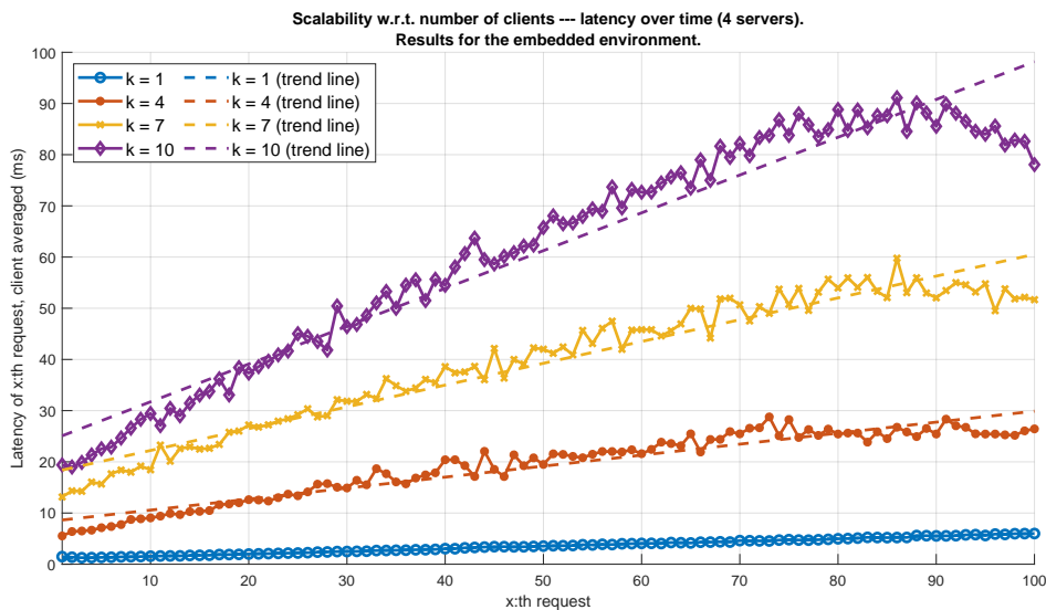
Figure 4.14: The result of Experiment 2 on the embedded environment. The x-axis is the x :th request. The y-axis is the latency in milliseconds. The bold lines are the measured latencies while the dashed lines are the corresponding trend lines, according to linear regression.
